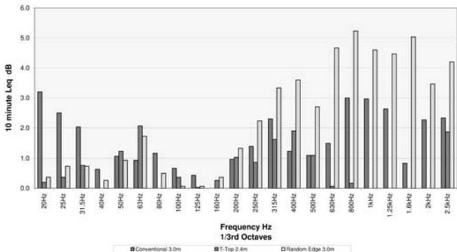
Figure 6: Comparison of spectral data of test barriers to the conventional 2.4m reference barrier at MPS
