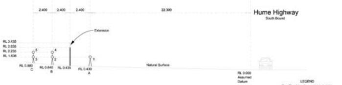
Figure 4: Cross section showing microphone positions A, B & C and barrier position
