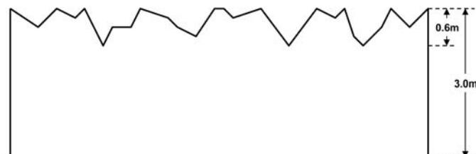
Figure 1: Representation of a random edge barrier used in the study
