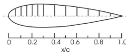
Figure 3. Pressure tap locations for unmodified airfoils
