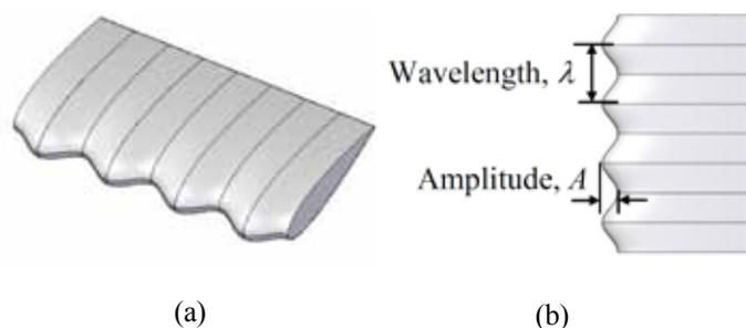
Figure 1. Section view of airfoil with tubercles (a) 3D view, (b) Plan view with characteristic dimensions
