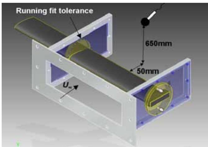
Figure 4. Mount for anechoic wind tunnel
