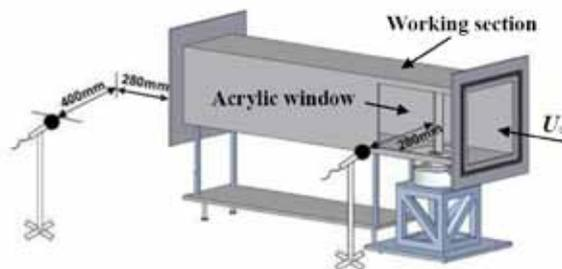
Figure 2. Working section and microphone positions
