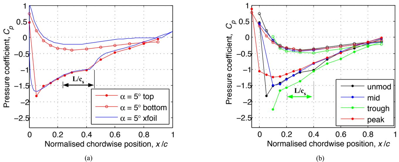
Figure 8. Normalised pressure distribution plots for (a) unmodified airfoil and (b) airfoil with A8230 tubercle configuration at  $\alpha = 5^\circ$ , where symbols are chosen as follows: “●” suction surface “○” pressure surface,  $Re = 120,000$ .
