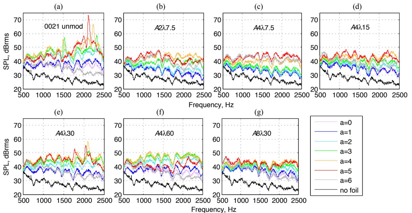
Figure 7. SPL against frequency measured in anechoic wind tunnel (AWT) for (a) unmodified 0021 (b)  $A2\lambda7.5$  (c)  $A4\lambda7.5$  (d)  $A4\lambda15$  (e)  $A4\lambda30$  (f)  $A4\lambda60$  (g)  $A8\lambda30$ ,  $Re = 120,000$
