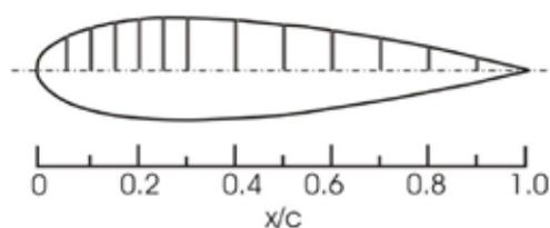
Figure 3. Pressure tap locations for unmodified airfoils
