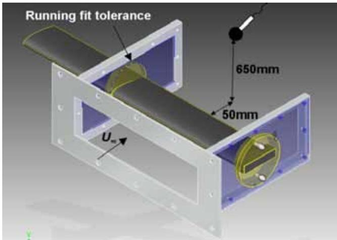
Figure 4. Mount for anechoic wind tunnel
