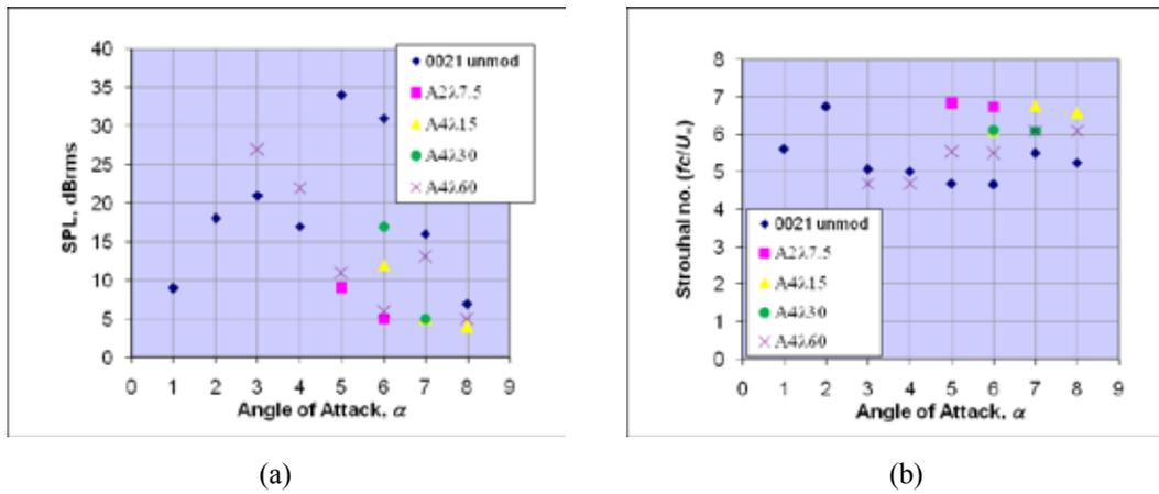
Figure 6. Results at microphone nearest window for NACA 0021 airfoils with tubercles at  $1^\circ \leq \alpha \leq 8^\circ$ . (a) Sound pressure level (SPL) against angle of attack,  $\alpha$  and (b) Strouhal number against angle of attack,  $\alpha$
