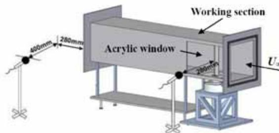
Figure 2. Working section and microphone positions
