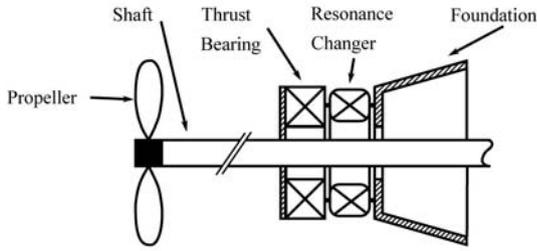
Figure 4. Propeller/shafting system
