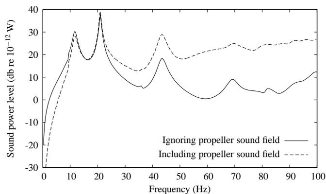
**Figure 12.** Sound power level for 1 N propeller force
