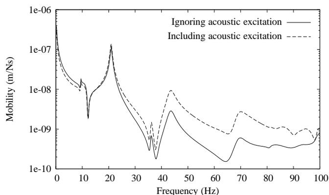
**Figure 11.** Mobility of the stern side end plate
