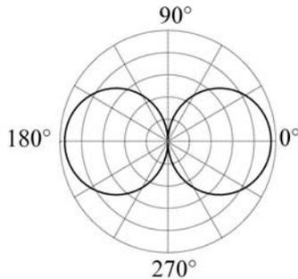
Figure 8. Dipole directivity pattern
