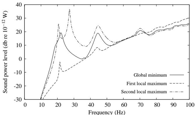
Figure 14. Sound power level for the minimum and maximum cost function values
