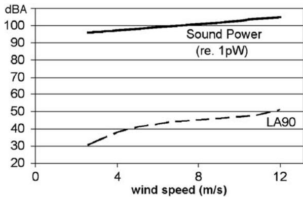
**Figure 1** LA90 measurements and reported sound power level at 125m from WTG tower versus wind speed at 10 m height.
