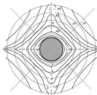
Figure 2. Wake of a torpedo [3]
