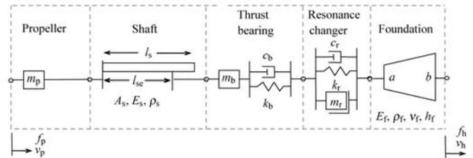
Figure 6. Modular approach for the propeller/shafting system [12]
