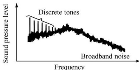
Figure 1. Non-cavitating noise of a submarine propeller [1]
