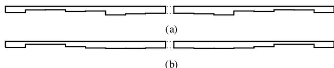
Figure 2: Profiles of circular plates with central hole (vertical scale distorted for clarity).
