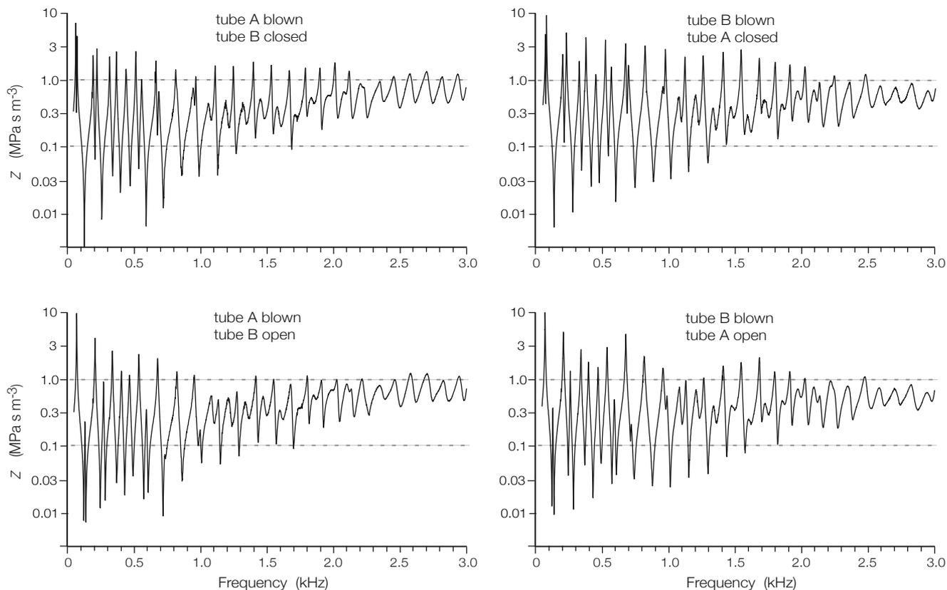
Figure 3. The measured acoustic input impedance  $Z_{IN}$  as a function of frequency plotted on a semi-logarithmic scale for the 4 possible input configurations of the forked didjeridu shown in Fig. 1.
