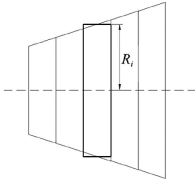
Figure 5. Local approximation of the conical shell.
