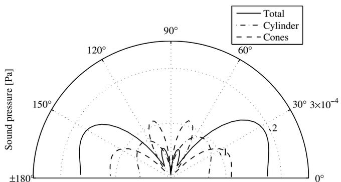
Figure 15. Directivity pattern at the second  $n=0$  natural frequency of 45.4 Hz.
