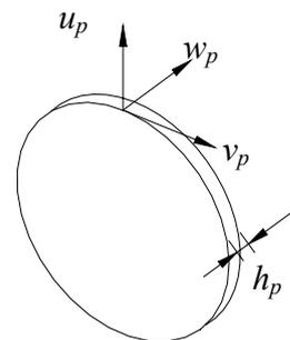
Figure 3. Displacements for a thin circular plate.
