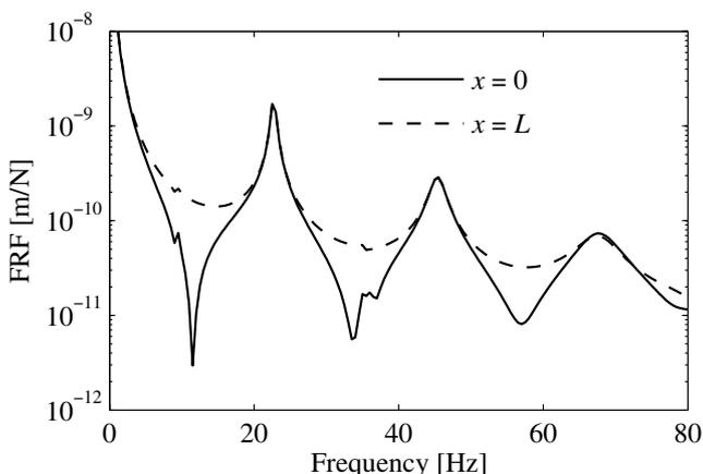
Figure 8. Frequency response of the axial displacement.
