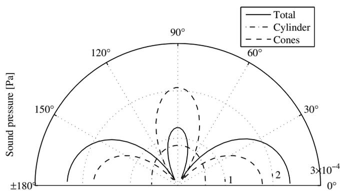
Figure 14. Directivity pattern at the first  $n=0$  natural frequency of 22.7 Hz.
