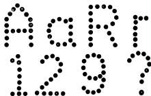
Fig. 5 Dot matrix representation of characters.
