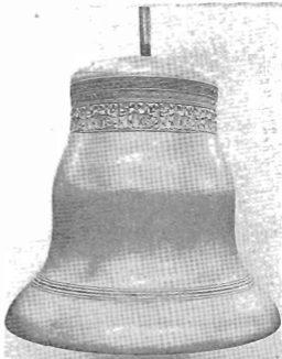
Figure 13: Probably the world's first true "major third" bell, produced in 1985 by the Royal Eijsbouts bell foundry, The Netherlands (bell diameter approx. 1000 mm, mass approx. 600 kg). (Photo courtesy Royal Eijsbouts)
