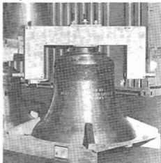
Figure 2: One bell from the electrically swung peal of six bells at Newcastle Cathedral, NSW (delivered 1977). This, the heaviest bell, has diameter 1010 mm, strike note g1 (252 Hz), and mass 540 kg. (Photo courtesy The Newcastle Morning Herald.)
