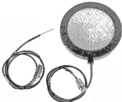
Figure 1: Needle (left) and membrane hydrophones. The active elements of both consist of the piezoelectric polymer PVDF. The element of the needle hydrophone is mounted at the end of the needle, perpendicular to the needle axis, and is approximately 0.5 mm in diameter. The active element of the membrane hydrophone is a poled spot approximately 0.5 mm in diameter at the centre of the membrane.
