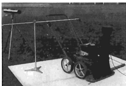
Figure 1. Billy Goat leaf sweeper with catenoidal horn on the inlet
