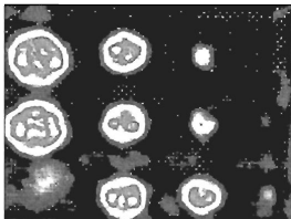
Figure 2. Pitch-Catch C-Scan of an impact damage test panel
