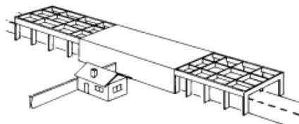
TUNNEL-WITH-HOLES TO CUT OUT NOISE
