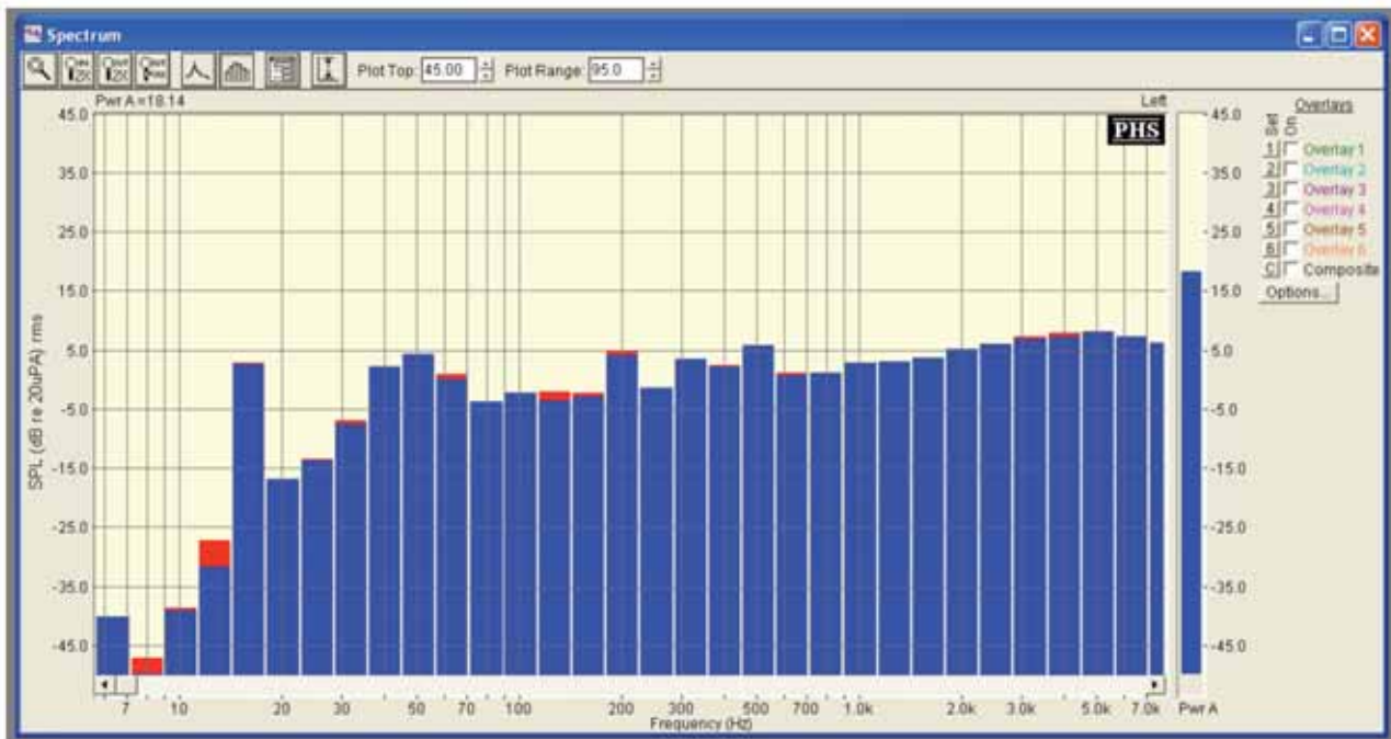
Figure 2. A-weighted third octave band spectrum in bedroom of house near a gold mine when the screens are in operation
