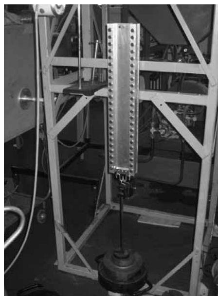
Figure 7. Photograph of the pull out experiment.
