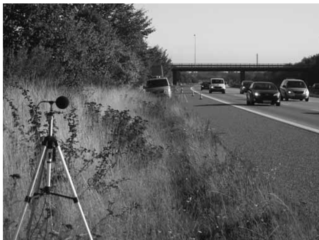
Figure 3: The Danish Road Institute measures the noise level at a test location for noise reducing pavement using the SPB method.
