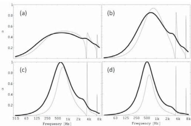
Figure 6. Effect of the hole diameter of the MPP of a porous layer-backed single MPP absorber. Thick line: porous layer-backed MPP; Thin line: air layer-backed MPP. Hole diameter  $d=0.1 \text{ mm}$  (a),  $0.2 \text{ mm}$  (b),  $0.5 \text{ mm}$  (c) and  $1.0 \text{ mm}$  (d). Thickness  $t=0.3 \text{ mm}$ , perforation ratio  $p=0.8\%$ , flow resistance of the absorbent  $R=10 \text{ kPa}\cdot\text{s}\cdot\text{m}^{-1}$  and cavity depth  $D=50 \text{ mm}$ .
