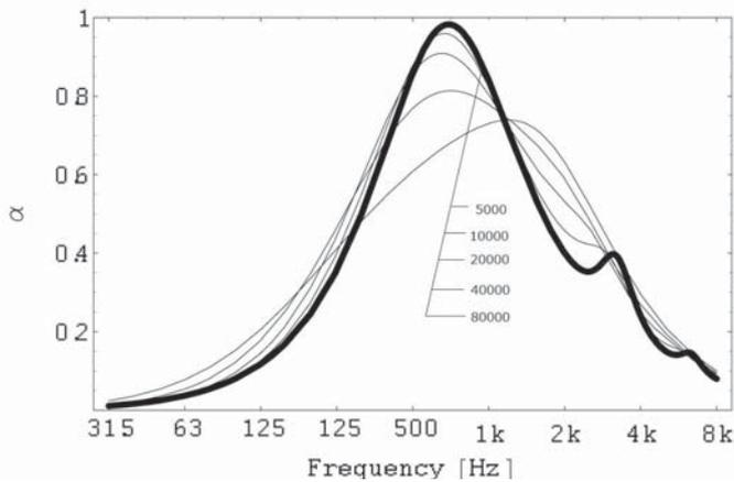
Figure 5. Effect of the flow resistance of the porous absorbent layer in the back cavity. Flow resistance of the absorbent  $R=5$  to  $80 \text{ kPa}\cdot\text{s}\cdot\text{m}^{-1}$ . Hole diameter  $d=0.3 \text{ mm}$ , thickness  $t=0.3 \text{ mm}$ , perforation ratio  $p=0.8\%$  and cavity depth  $D=50 \text{ mm}$ .
