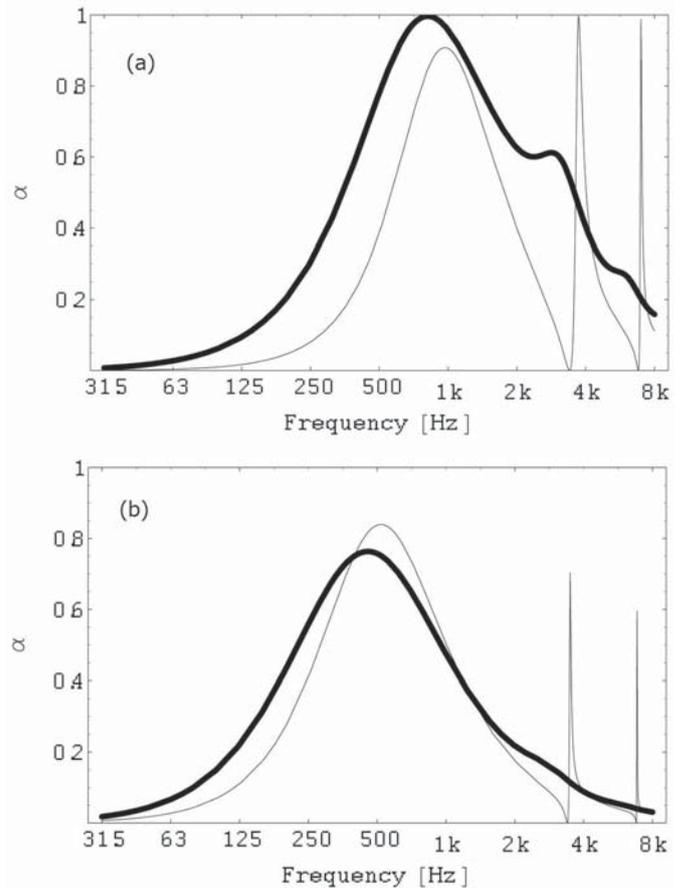
Figure 7. Effect of the thickness of the MPP of a porous layer backed single MPP absorber. Thick line: porous layer backed MPP; Thin line: air layer backed MPP. Thickness  $t=0.1 \text{ mm}$  (a), and  $1.0 \text{ mm}$  (b). Hole diameter  $d=0.3 \text{ mm}$ , perforation ratio  $p=0.8\%$ , flow resistance of the absorbent  $R=10 \text{ kPa}\cdot\text{s}\cdot\text{m}^{-1}$  and cavity depth  $D=50 \text{ mm}$ .
