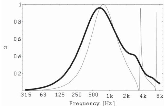
Figure 4. Comparison of the absorption characteristics of an MPP absorber backed by an air cavity (thin line) and that backed by a porous absorbent layer (thick line). Hole diameter  $d=0.3$  mm, thickness  $t=0.3$ mm, perforation ratio  $p=0.8\%$ , flow resistance of the absorbent  $R=10$  kPa.s.m<sup>-1</sup> and cavity depth  $D=50$  mm
