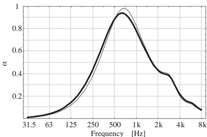
Figure 3. Comparison of the absorption coefficient using the impedance derived from the present theory and Maa's theory in the porous layer-backed case.  $d=t=0.3$  mm,  $p=0.8\%$ ,  $D=50$  mm,  $R=10$  kPa.s.m<sup>-1</sup>. Thick line: the present theory, Eqs. (24) to (26); Thin line: Maa's theory, Eqs. (1) and (2)
