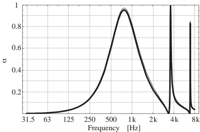
Figure 2. Comparison of the absorption coefficient using the impedance derived from the present theory and Maa's theory in the air-backed case:  $d=t=0.3$  mm,  $p=0.8\%$ ,  $D=50$  mm. Thick line: derived by the present theory, Eqs. (21) to (23); Thin line: Maa's theory, Eqs. (1) and (2)
