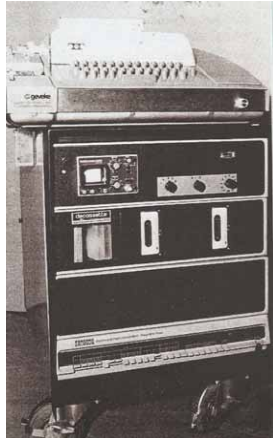
Figure 2. STIDAS I (STI Device using Artificial Signals) device based on a PDP-11/10 computer and custom analog hardware (1971)
