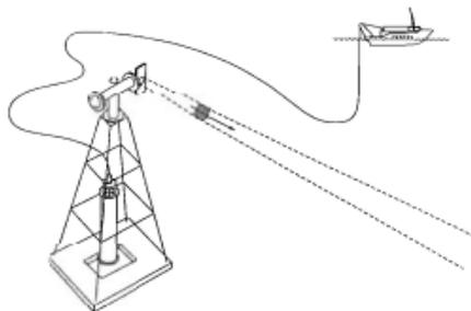
Figure 1. Arrangement of tower on sea floor, showing umbilical to surface.
