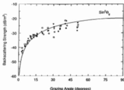
Figure 3. Bottom backscattering strength, frequency 100 kHz, shallow site N1, tower measurement.
