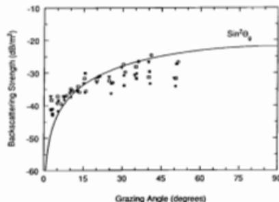
Figure 4. Bottom backscattering strength, frequency 200 kHz, deep site N1, tower measurement.
