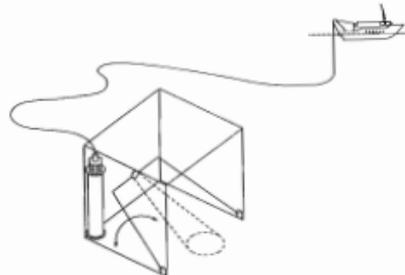
Figure 2. Arrangement of frame on sea floor, showing umbilical to surface.
