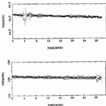
Figure 4. Application of the PIE method to real passive sonar data. The fundamental (first harmonic) and third harmonic of a nominally 45 Hz acoustic projector are plotted as a function of time. Sampling rate was 470.7 Hz and the FFT resolution was 0.46 Hz.
