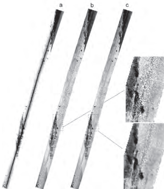
Figure 6. EM300 backscatter for a vessel track at \sim 200 m depth for (a) raw, (b) backscatter referenced to 1000 ping average at 40^\circ incidence angle to the seabed, (c) after low pass filtering. Dynamic range is -20 dB dark and -40 dB light. The inserts highlight the effects of the median 3 beams by 3 pings box car filter on the backscatter
