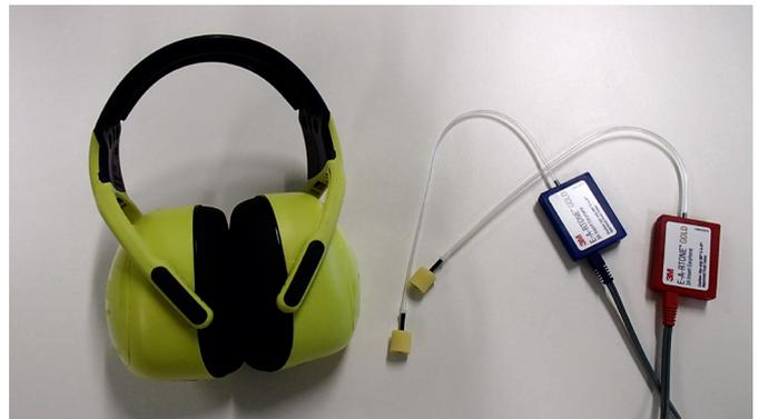
Figure 1. MSA 766243 High Profile Earmuff and ER-3A insert earphones
