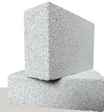
Reapor® panels are NRC.90@50mm. Non-combustible Group 1 fire rating, resistant to weather or pollution aging, simply adhesive fixed, cut with normal wood working equipment.
