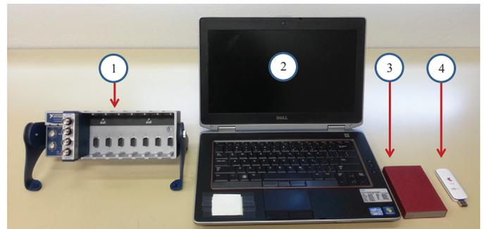
Figure 1. Set up for Remote Data Acquisition System
