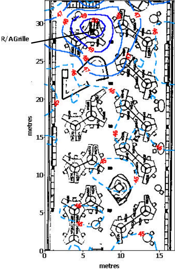
Figure 4 Spatial coverage of Level 11 South wing, showing return air (R/A) grille 'hot spots'. Contour values = 1 dBA.
