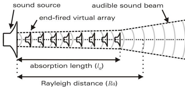
Figure 2. Schematic of the parametric array.
