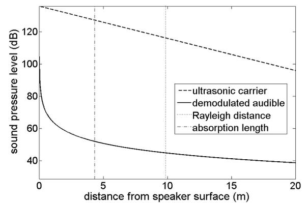
Figure 3. On-axis sound pressure level of the ultrasonic carrier and demodulated fundamental frequency for a 130 dB ultrasonic source modulated with a 500 Hz tone.
