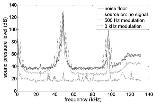
**Figure 11.** Frequency response of the parametric array.
