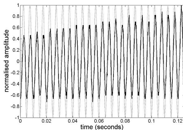
**Figure 8.** Time trace of the normalised input modulation signal (.....) and the normalised demodulated signal recorded at a distance of 1 metre from the source (—) for a 200 Hz modulation signal.
