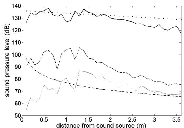
**Figure 6.** On-axis sound pressure level of the ultrasonic carrier (—), fundamental audible demodulated frequency (---), and the first harmonic of the demodulated frequency (···) for a modulation frequency of 1 kHz. The theoretical approximations of the ultrasonic carrier (· · ·) and demodulated fundamental frequency (---) are also shown for comparison.
