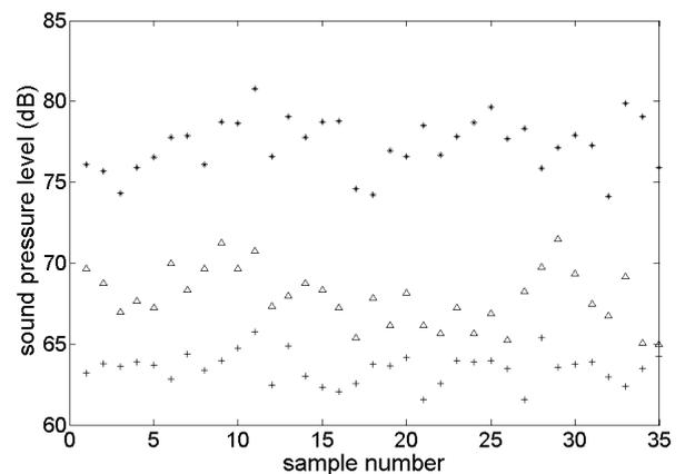
**Figure 9.** Temporal variation in SPL at frequencies of 250 Hz (Δ), 1 kHz (\*) and 5 kHz (+).
