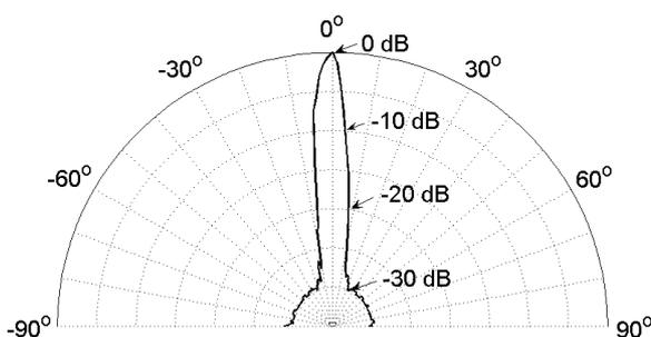
**Figure 4.** Directivity of a 500 Hz signal at a distance of 1.5 m from the parametric array.
