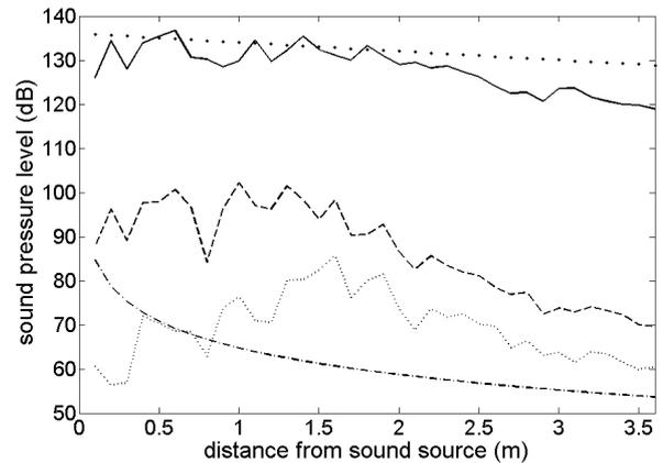
**Figure 5.** On-axis sound pressure level of the ultrasonic carrier (—), fundamental audible demodulated frequency (---), and the first harmonic of the demodulated frequency (···) for a modulation frequency of 500 Hz. The theoretical approximations of the ultrasonic carrier (· · ·) and demodulated fundamental frequency (---) are also shown for comparison.
