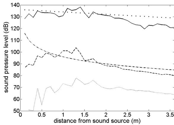
**Figure 7.** On-axis sound pressure level of the ultrasonic carrier (—), fundamental audible demodulated frequency (---), and the first harmonic of the demodulated frequency (.....) for a modulation frequency of 3 kHz. The theoretical approximations of the ultrasonic carrier (· · ·) and demodulated fundamental frequency (---) are also shown for comparison.
