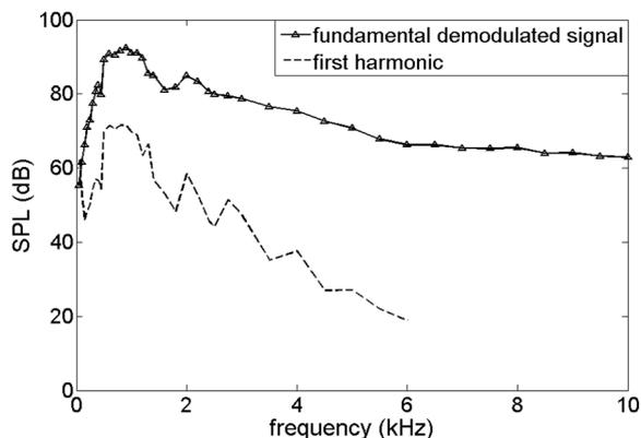
**Figure 10.** SPLs of the fundamental demodulated signal and its first harmonic as a function of frequency.
