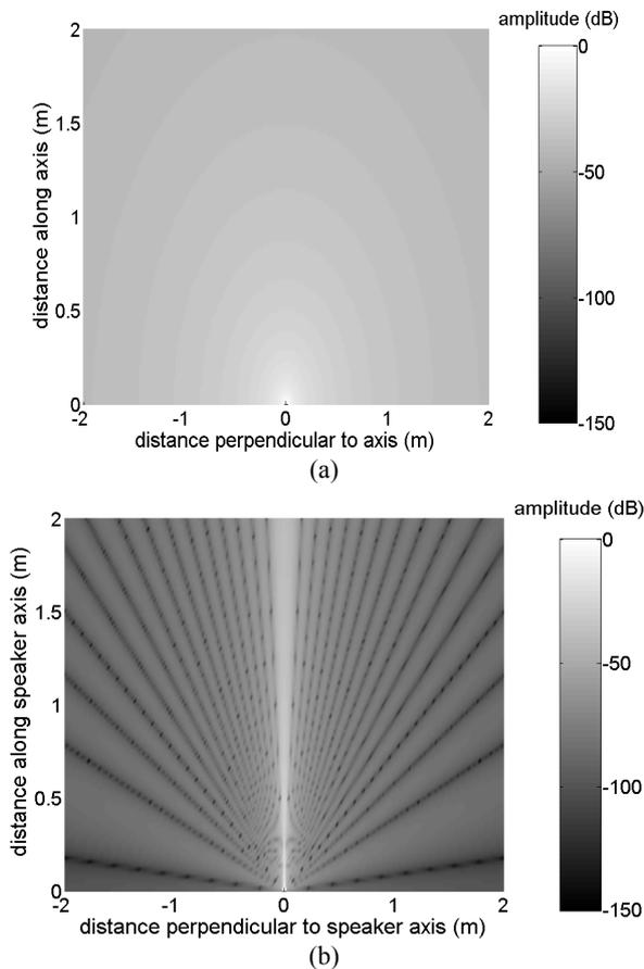
**Figure 1.** Comparison between directivity of a) a single source emitting sound at 500 Hz to b) a source emitting sound at 48 kHz.
