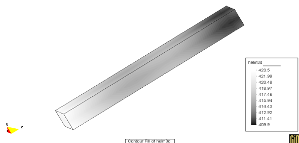
Figure 8. Travelling wave in a duct (pressure in Pascals).
