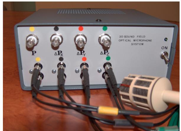
(b) Sensor head and electro-optical unit
