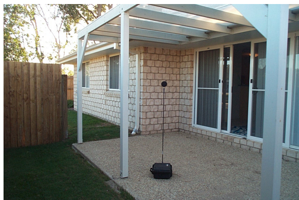
Figure 4. Noise Logger Behind the Screen
