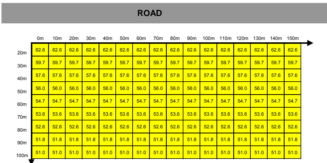
Figure 8. Grid for two-dimensional road traffic noise predictions. L_{eq} values are for a speed of 80 km/h.
