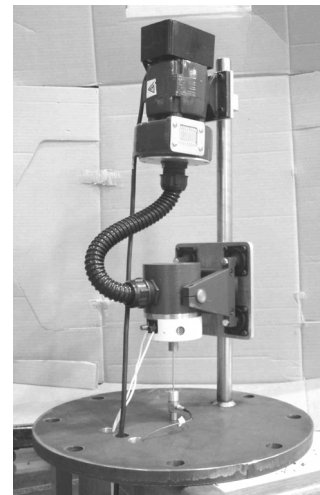
Figure 3. The driven end plate, showing (top to bottom) the blower, shaker, stinger and force transducer at the centre of the plate. Access for leads is by three extra holes in the plate.
