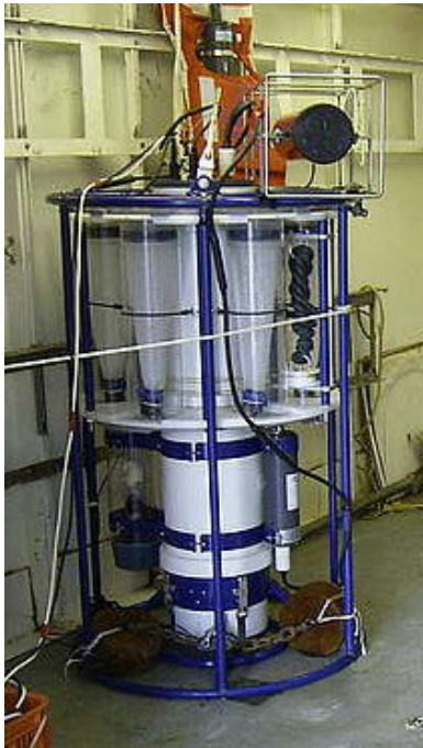
Figure 1. The specially designed Discreet In-situ Plankton Sampler (DIPS) that can collect 6 samples at targeted water depths and the Tracor multi-frequency (TAPS) acoustic system attached.
