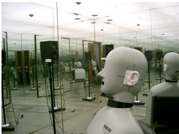
Figure 9. HATS impulse response measurements in the artificial sky lab (room 1).
