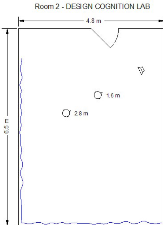
Figure 5. Listening test set-up in room 2 (second loudspeaker).
