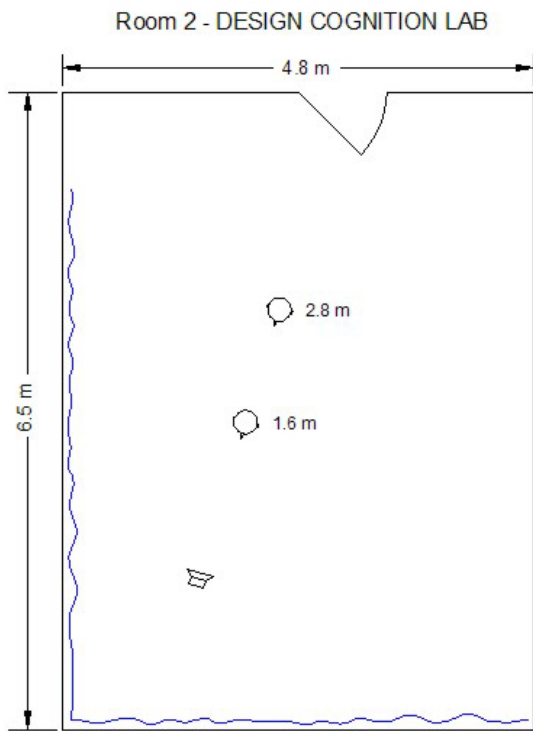
Figure 4. Listening test set-up in room 2 (first loudspeaker).
