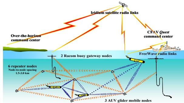
**Figure 4.** The February 2003 Q272 Seaweb network in the Eastern Gulf of Mexico included three AUVs, six repeater nodes, and two gateway buoys. The experiment exercised Seaweb ranging functions for tracking and navigating mobile nodes. The AUVs proved themselves as effective mobile gateway nodes with telesonar, FreeWave, Iridium, ARGOS, and GPS.
