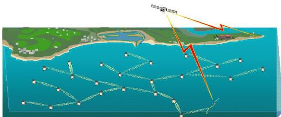
**Figure 1.** Seaweb through-water acoustic networking enables data telemetry and remote command & control for undersea sensor grids, autonomous instruments, and vehicles.
