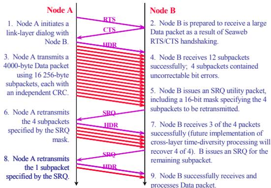
**Figure 3.** Selective ARQ (SRQ) is a link-layer mechanism for reliable transport of large data files between neighboring nodes even when the physical layer suffers bit errors uncorrectable by forward error correction, as depicted in the example here. Purple arrows are Seaweb utility packets. Red arrows are data sub-packets.
