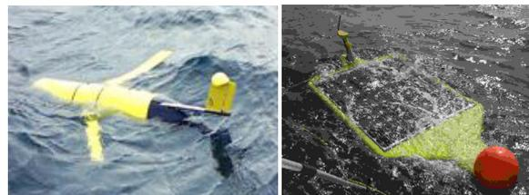
**Figure 5.** Left: SLOCUM gliders are buoyancy-driven mobile Seaweb nodes for which acoustic sensors and towed arrays are now being developed. Telesonar transducer in the nose section, combined with GPS, Iridium, FreeWave, and ARGOS in the tail make these AUVs effective mobile gateway nodes without the attendant vulnerability of moored gateways. Right: SAUV is a solar-powered propeller-driven AUV with a virtually unlimited life. SAUV is also fitted with telesonar, Iridium, FreeWave, and GPS.
