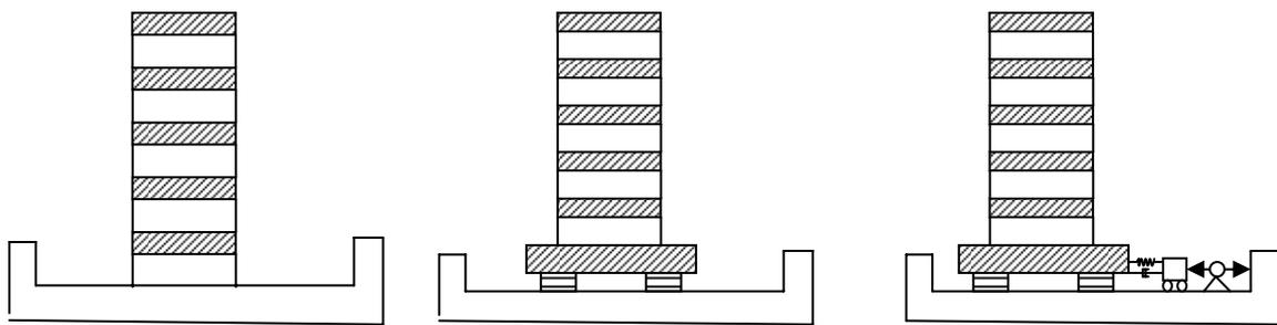
(a) Bare frame (b) Base isolated frame (c) Hybrid controlled frame
