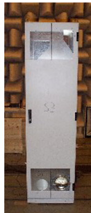
Figure 2 A telecommunications base station with cooling fans in the door (from Moorhouse et. Al. 2003)
