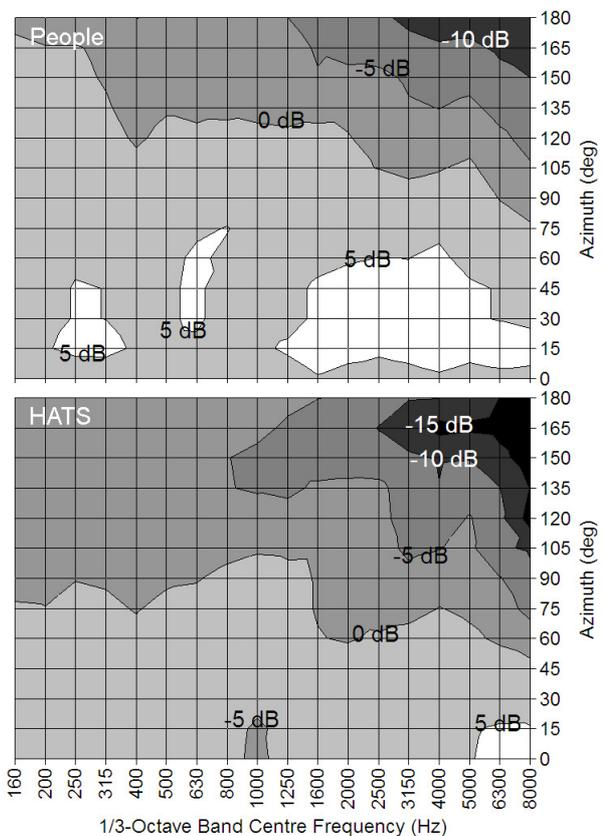
**Figure 6.** Measured directivity index of people speaking, and of a head and torso simulator (HATS) as a function of frequency and angle of rotation (based on Chu and Warnock, 2002).
