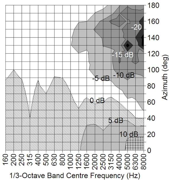
Figure 7. Measured directivity index of an NTI Talkbox as a function of frequency and angle of rotation.
