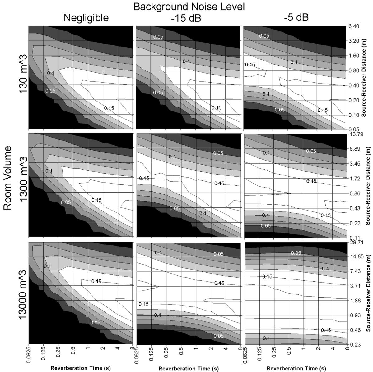
**Figure 3.** Standard deviation of STI for a range of source directivity factors ( $Q_s$ ) from 0.125 to 8, for the case of constant power. Results are shown as a function of reverberation time, source-receiver distance, room volume and background noise relative to anechoic speech at 1 m when  $Q_r = 1$ .
