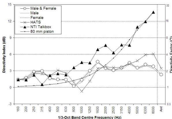
**Figure 5.** On-axis directivities of human talkers and a Bruel & Kjaer 4128C head and torso simulator, derived from Chu and Warnock’s (2002) data; and the measured on-axis directivity of an NTI Talkbox, compared with the expected value for an 80 mm circular piston on the end of a long cylinder.
