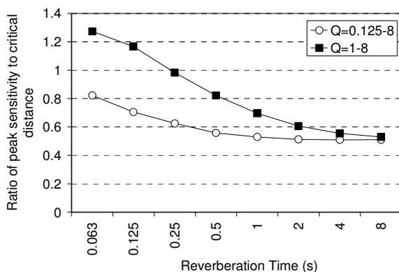
Figure 8. The distance of peak sensitivity to source directivity divided by the critical distance as a function of reverberation time. Two ranges of directivities are evaluated:  $Q_t = 0.125 - 8$ ; and  $Q_t = 1-8$ .
