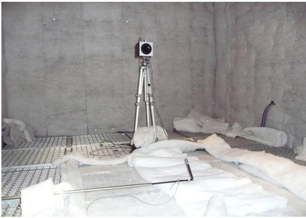
**Figure 4.** NTI Talkbox directivity measured using Bruel & Kjaer Electro-acoustic Pulse System Type 7907 with turntable in Anechoic Chamber
