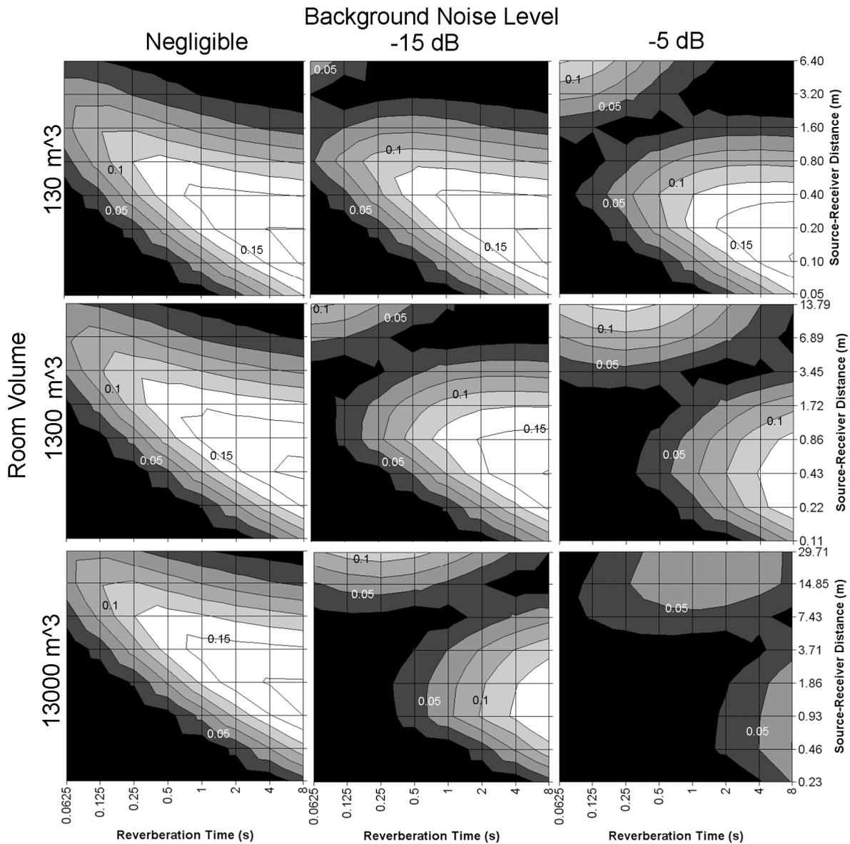
**Figure 2.** Standard deviation of STI for a range of source directivity factors ( $Q_s$ ) from 0.125 to 8, for the case of constant on-axis sound pressure. Results are shown as a function of reverberation time, source-receiver distance, room volume and background noise relative to anechoic on-axis speech at 1 m.
