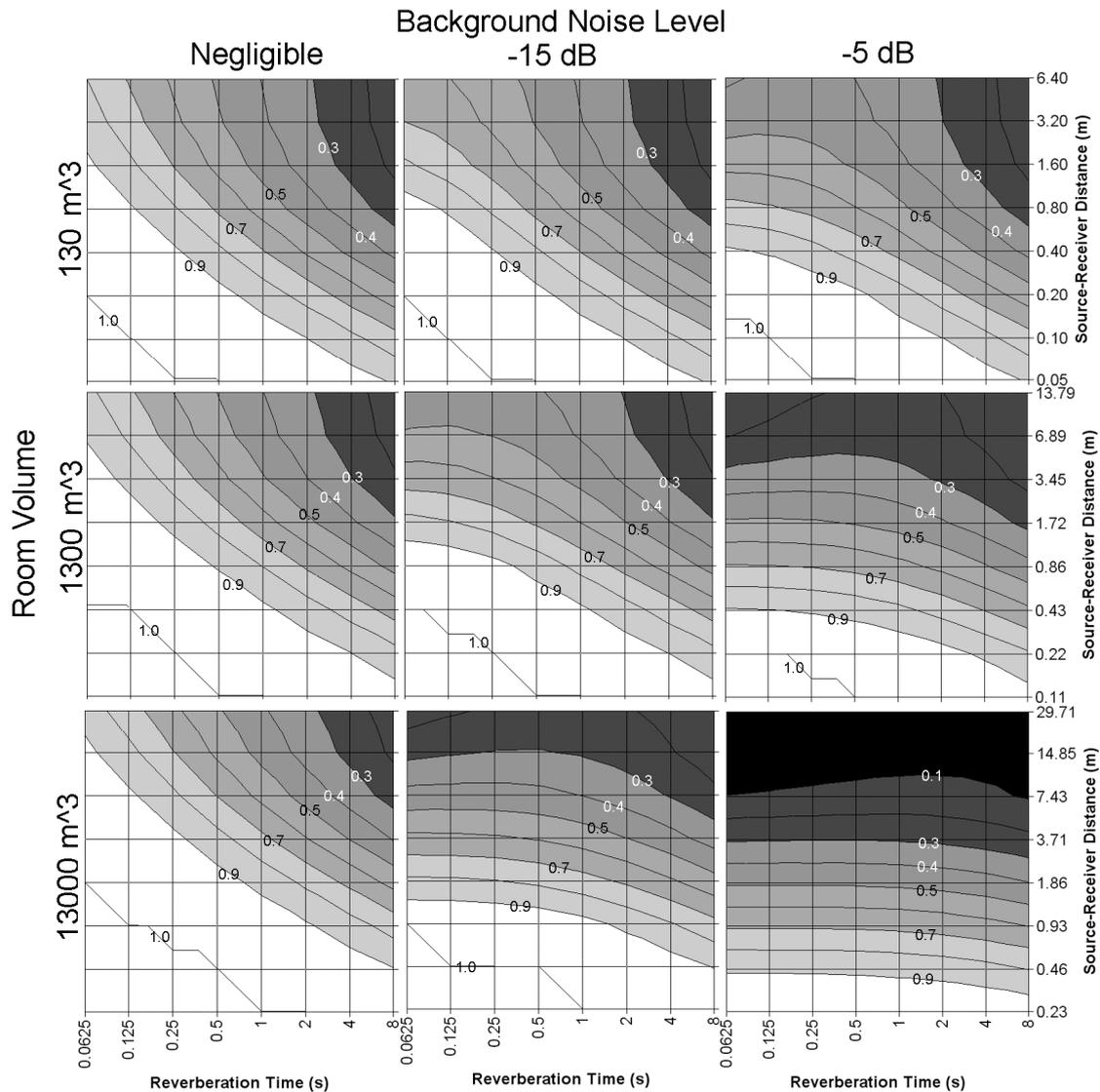
**Figure 1.** Mean STI for a range of source directivity factors ( $Q_s$ ) from 0.125 to 8. Results are shown as a function of reverberation time, source-receiver distance, room volume and background noise relative to anechoic on-axis speech at 1 m. While values are for the case of constant on-axis pressure, almost identical values are found for the case of constant source power.
