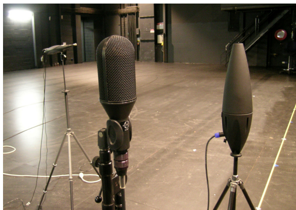
Figure 3. Left is the B & K measurement mic, Centre is the Soundfield mic and Right is the Tulip, omnisource speaker.
