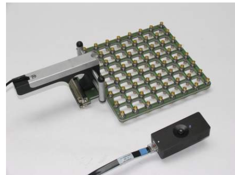
Figure 4 Example of a handheld array with ultrasonic transducers for detecting array position
