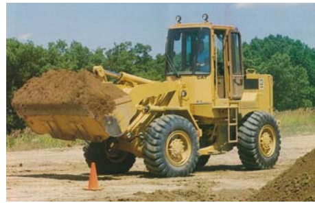
Figure 2. Front end loader
