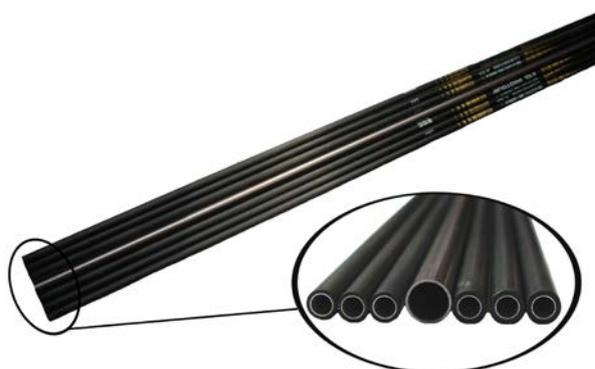
**Figure 3.** Archery arrow specimens, pictured from left to right the ProTour570, Superlite1713 and ProTour380.
