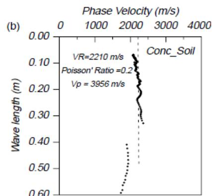
Figure 6: Concrete slab Dispersion Curve example (Kim, D. S., W. S. Seo, et al., 2006)
