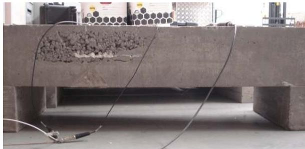
Figure 14: Single layer concrete sample with honeycomb flaw
