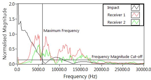
Figure 13: Experimental SASW Data Frequency Spectrum
