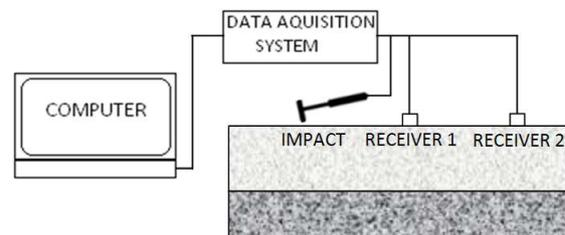
Figure 5: SASW test configuration
