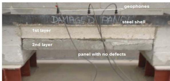
Figure 15: Layered concrete test sample with no defects
