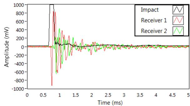
Figure 12: Experimental SASW Data Time Signal
