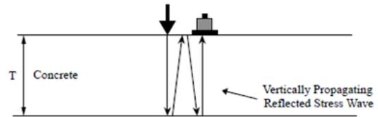
Figure 4: Impact echo test configuration (Kim, Seo et al., 2006)
