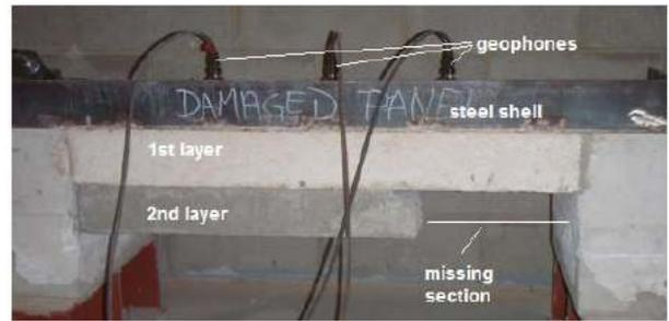
Figure 16: Layered concrete test sample with void
