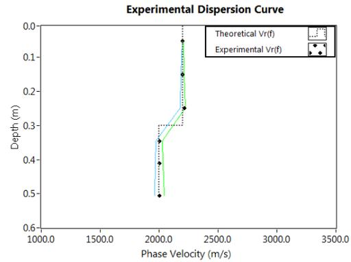
Figure 11: Two layer artificial data dispersion curve (with error bands)
