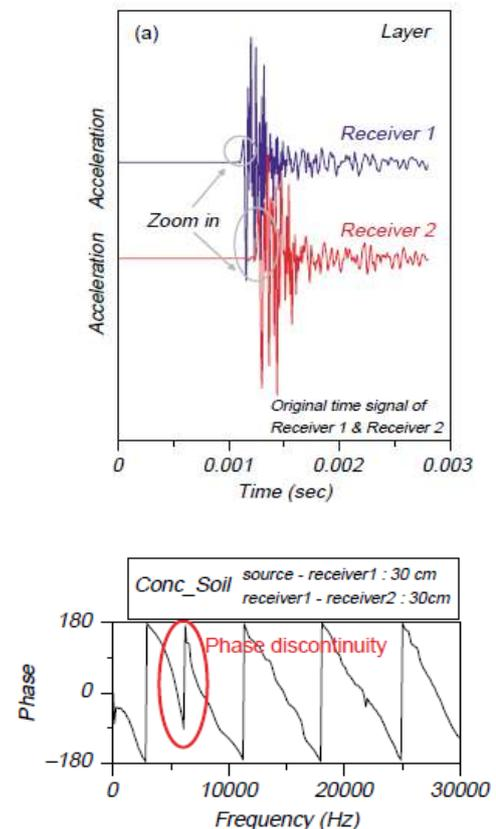
Figure 2: Phase difference between receiver signals (Kim, Seo, et al., 2006)
