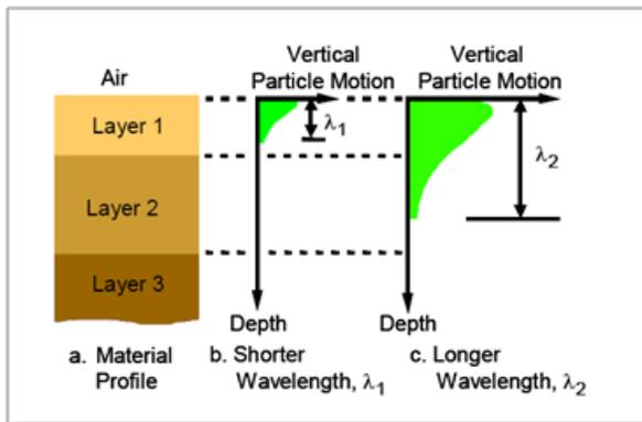
Figure 3: Rayleigh wave motion (Geovision, 2010)
