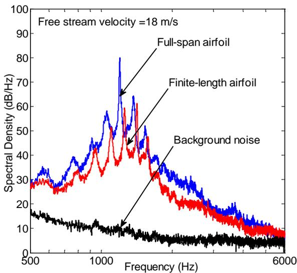
Figure 7: Airfoil self noise at  $Re_c = 8 \times 10^4$  ( $\alpha^* = 0^\circ$ )
