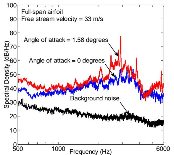
Figure 13: Airfoil noise spectra at  $Re_c = 1.53 \times 10^5$
