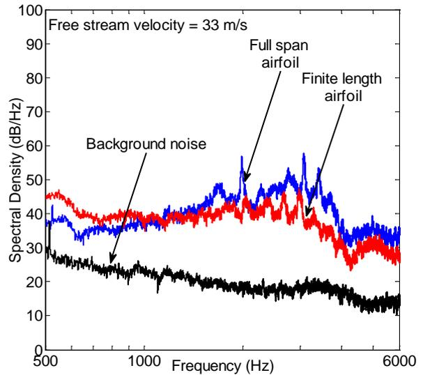
Figure 8: Noise spectrum at  $Re_c = 1.31 \times 10^5$  ( $\alpha^* = 0^\circ$ )
