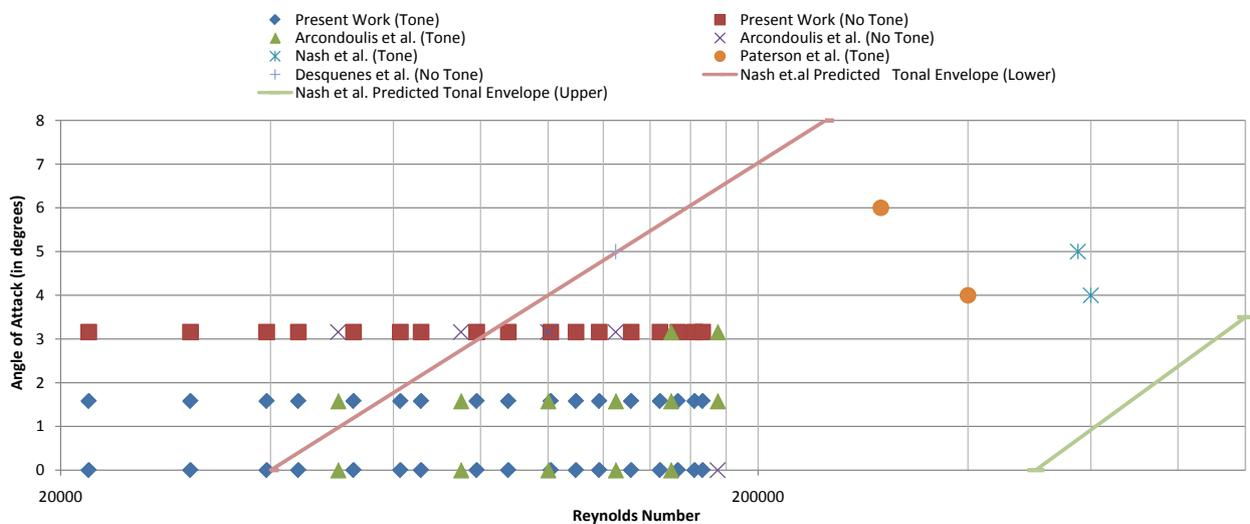
Figure 21: Tonal envelope predicted by Nash et al.(1999)
