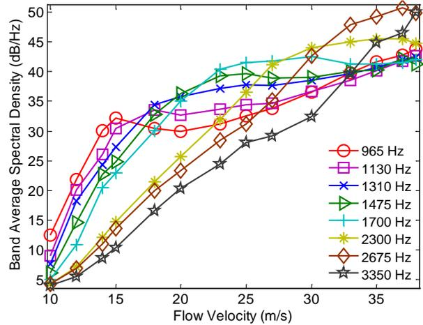
**Figure 17:** RMS of spectral density vs flow velocity (Finite-length airfoil at  $1.58^\circ$  angle of attack)
