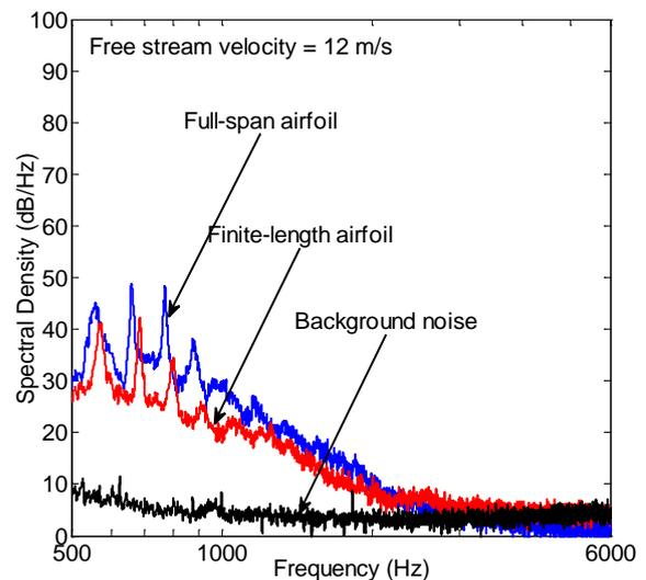
Figure 9: Noise spectra for  $Re_c = 5.26 \times 10^4$  ( $\alpha^* = 1.58^\circ$ )
