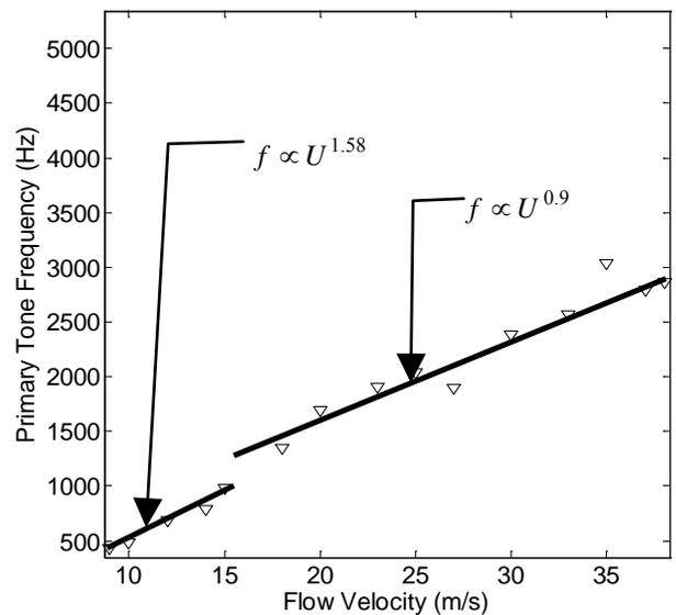
Figure 20: Frequency of the primary tones vs flow velocity for airfoil at  $\alpha^* = 1.58^\circ$
