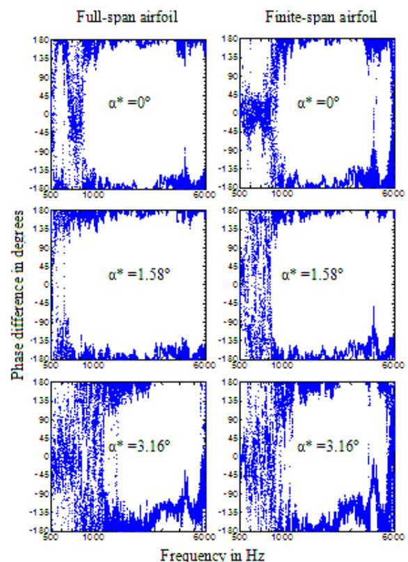
Figure 5: Phase difference between top and bottom microphone noise data at  $Re_c = 1.675 \times 10^5$
