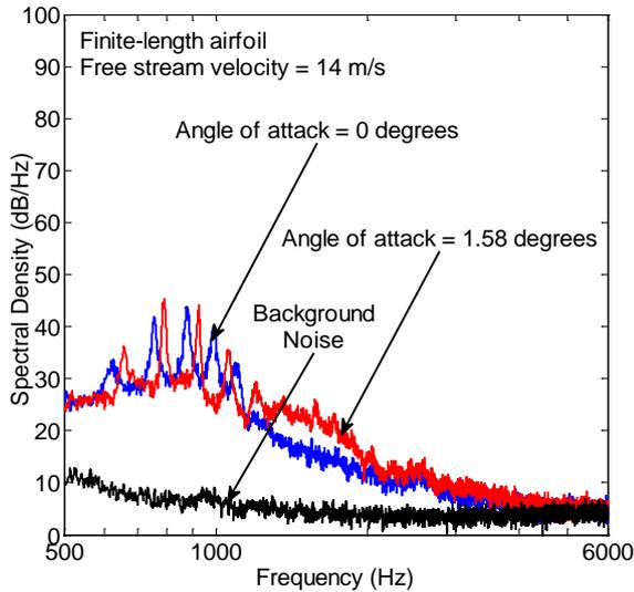
Figure 10: Noise spectra at  $Re_c = 6.14 \times 10^4$
