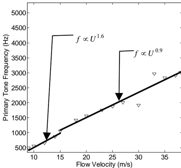
Figure 19: Frequency of the primary tones vs flow velocity for airfoil at  $\alpha^* = 0^\circ$
