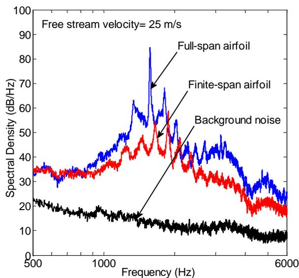
Figure 4: Noise spectra at  $Re_c = 1.1 \times 10^5$
