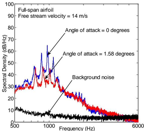
Figure 11: Noise spectra at  $Re_c = 6.14 \times 10^4$
