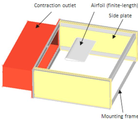
Figure 2: Airfoil in test condition ( $\alpha^* = 0^\circ$ )
