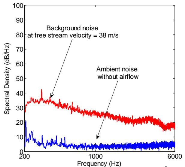
Figure 3: Background noise at  $Re_c = 1.67 \times 10^5$  (flow velocity 38 m/s)
