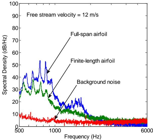
Figure 6: Noise spectra at  $Re_c = 5.26 \times 10^4$  ( $\alpha^* = 0^\circ$ )
