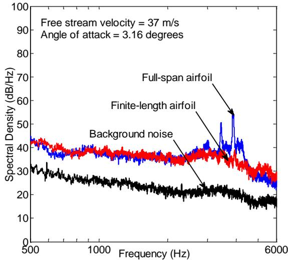
**Figure 15:** Noise spectra at  $Re_c 1.63 \times 10^5$
