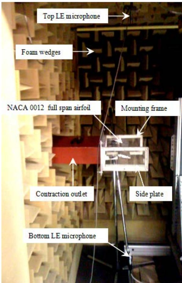
Figure 1: Experimental setup ( $\alpha^* = 3.16^\circ$ )
