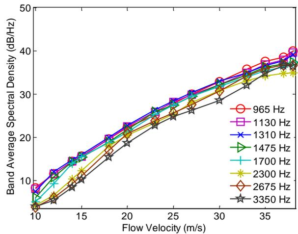
**Figure 18:** RMS of spectral density vs flow velocity (Finite-length airfoil at  $3.16^\circ$  angle of attack)
