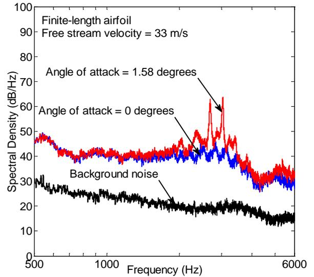
Figure 12: Noise spectra at  $Re_c = 1.53 \times 10^5$
