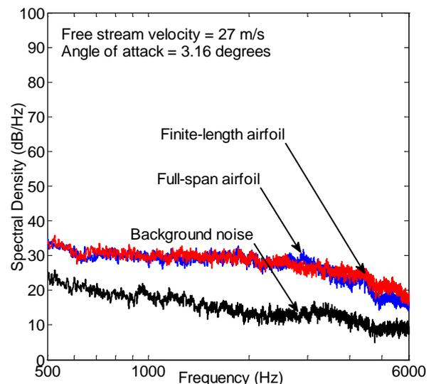
Figure 14: Noise spectra at  $Re_c = 1.18 \times 10^5$
