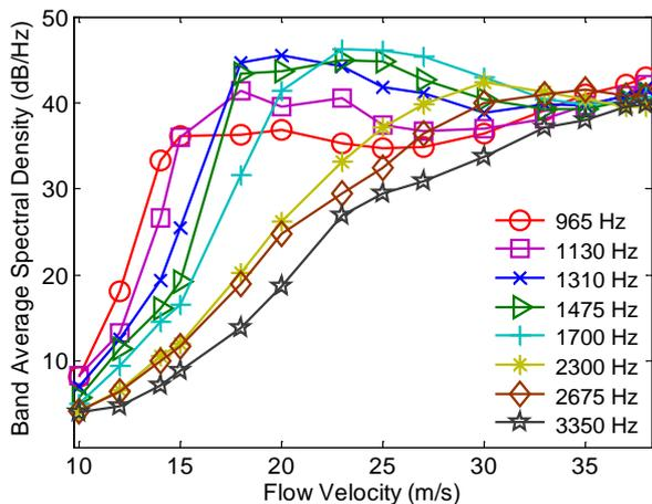
**Figure 16:** RMS of spectral density vs flow velocity (Finite-length airfoil at  $0^\circ$  angle of attack)
