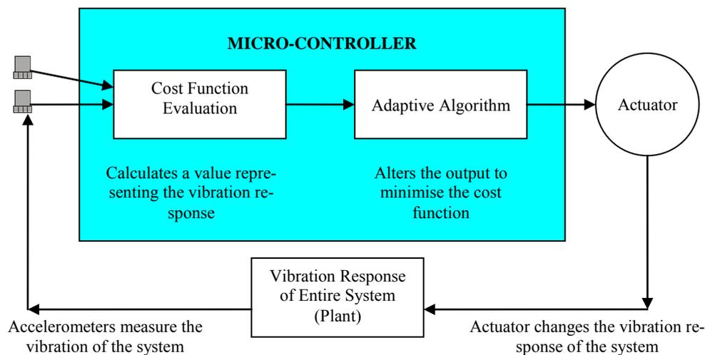
Figure 1: Adaptive-passive control system.
