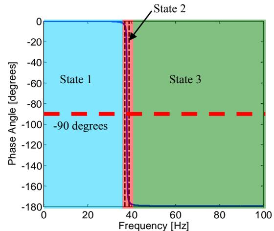
**Figure 3:** Definition of system states based on the phase angle of the TVN.
