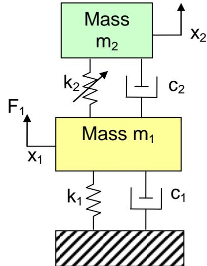
**Figure 2:** Model of an adaptive tuned vibration neutraliser attached to a vibrating primary structure.
