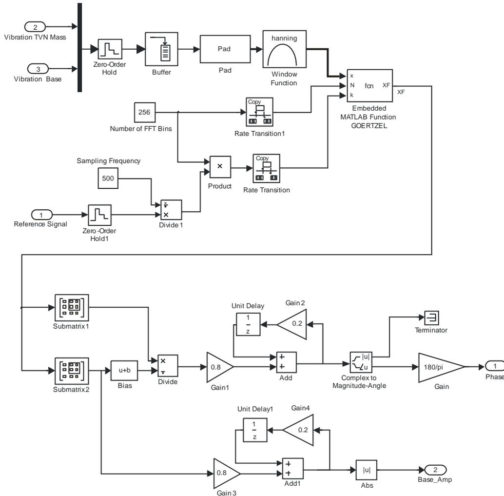
Figure 4: Simulink model to calculate the 'cost function' that uses the Goertzel algorithm.
