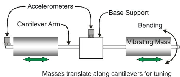
Figure 5: Adaptive tuned vibration neutraliser comprising masses on cantilever arms.
