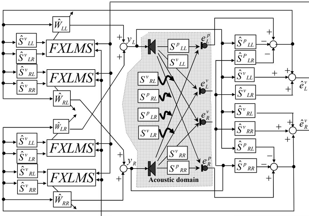
Figure 4 Active headrest algorithm using virtual microphone arrangement.
