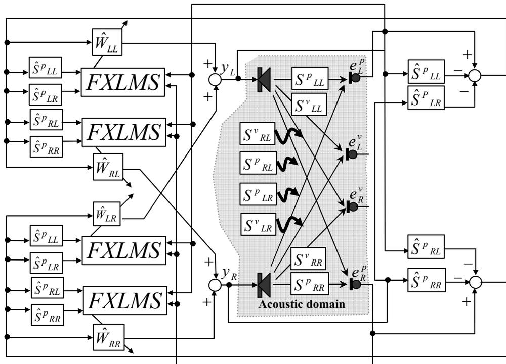
Figure 3 Active headrest algorithm controlling noise at physical microphones.
