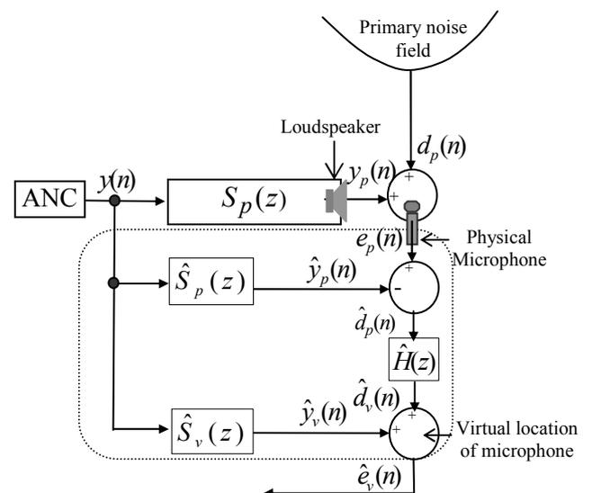
Figure 1 Remote microphone technique for estimating virtual error signal
