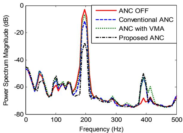
**Figure 7** The power spectrum magnitude of the microphone signal placed at the left ear of the manikin.
