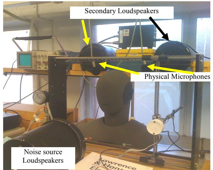
**Figure 5** Experimental setup for active headrest (a) schematic diagram (b) photograph.
