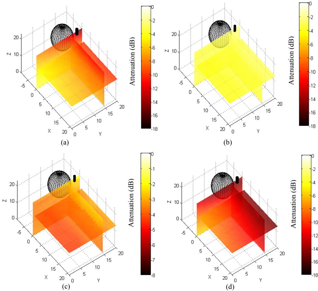
**Figure 6** Noise attenuation profile on the left side of the head in three orthogonal planes crossing near the ear (a) Conventional ANC with physical microphone control (b) ANC with VMA Technique (c) ANC with VMA Technique (lower scale) (d) Proposed ANC with RMT. The sphere represents the position of the head, and the cylinder the physical microphone.
