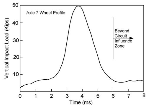
**Figure 6.** A typical impact due to a wheel/rail out-of-round defect (1 kip = 4.448 kN)
