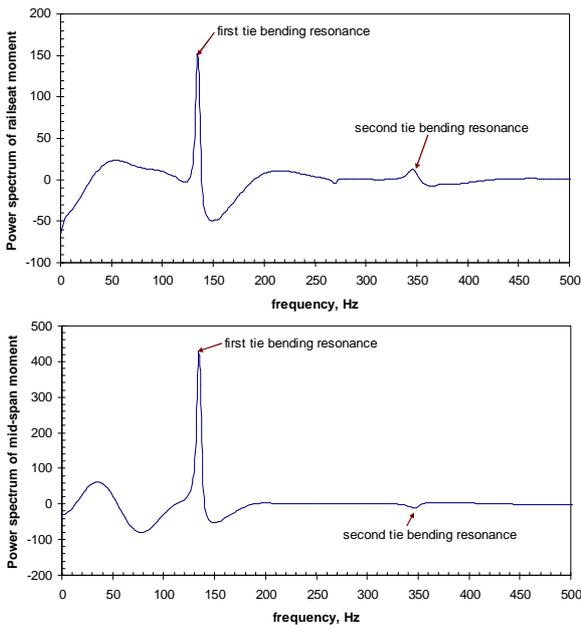
**Figure 16.** Transient responses of evenly supported railway concrete sleeper to sinusoidal pulse in frequency domain
