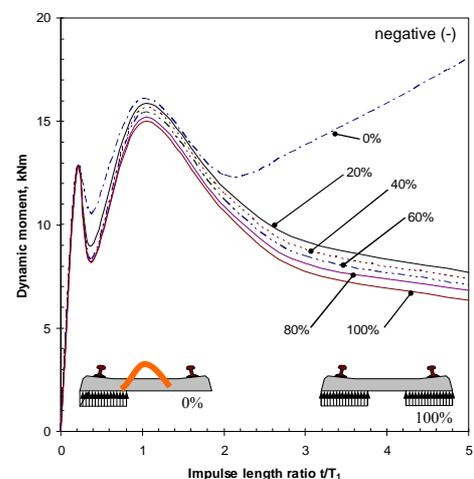
**Figure 18.** Dynamic bending moments at the right-hand-side rail seat of voided sleepers to impact loading
