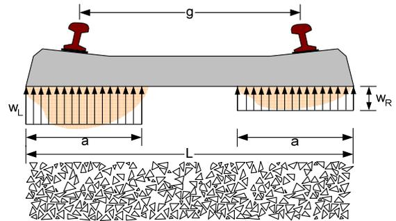
**Figure 5.** Asymmetrical ballast stiffness distribution
