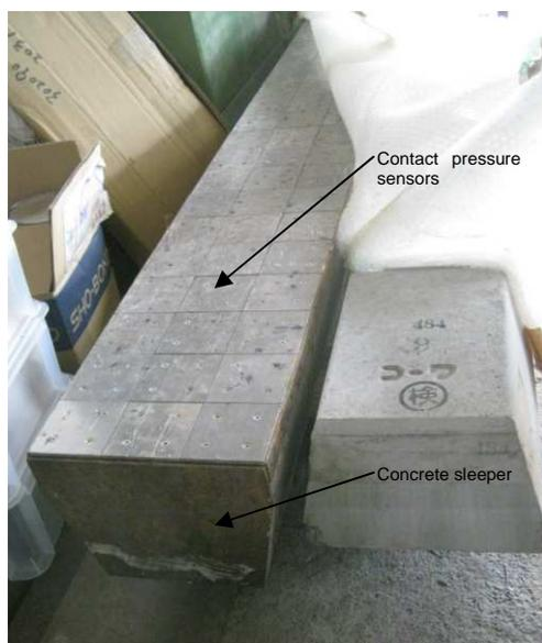
Figure 20. Instrumented sleepers
