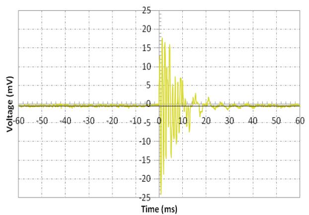
Figure 12. Solid timber rubber ball test differential output.
