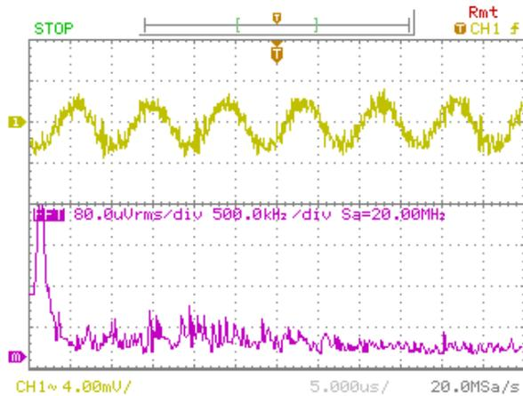
Figure 13. Ceramic tile response to 108.5 KHz signal
