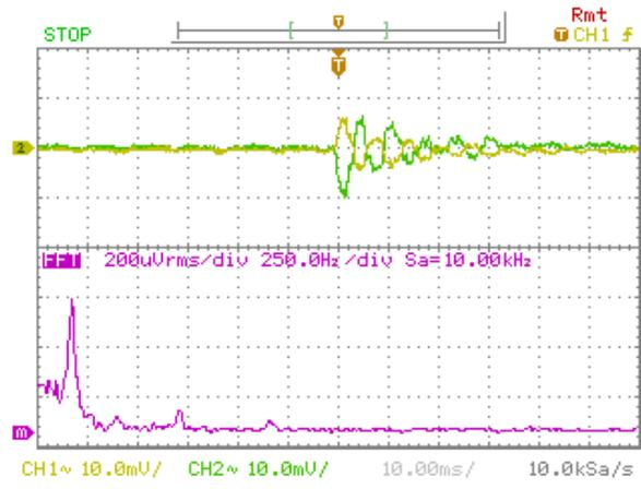
Figure 10. Porcelain composite tile low velocity impact test.
