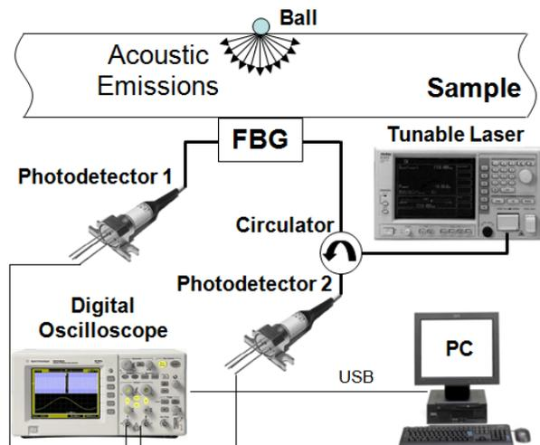
**Figure 5.** Setup for the AE experiments
