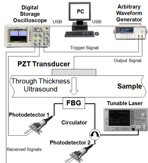
**Figure 6.** Setup for the actively generated acoustic signals.
