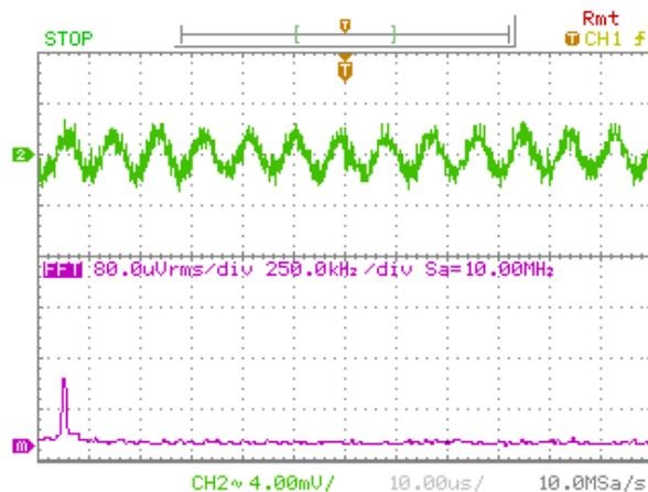
Figure 14. Aluminium response to 112.2 KHz signal.
