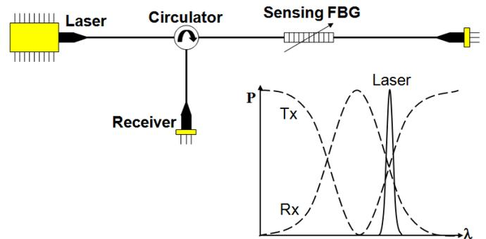
Figure 2. Optical circuit of the TRDS, with the tunable laser (TL), and the transmit (Tx) and reflect (Rx) receivers. The inset shows the spectrum of the optical components
