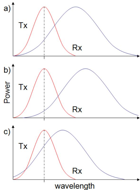
Figure 3. Operating principle of the TRDS, a) shows the FBG with no change in measurand, b) a positive change, and c) a negative change
