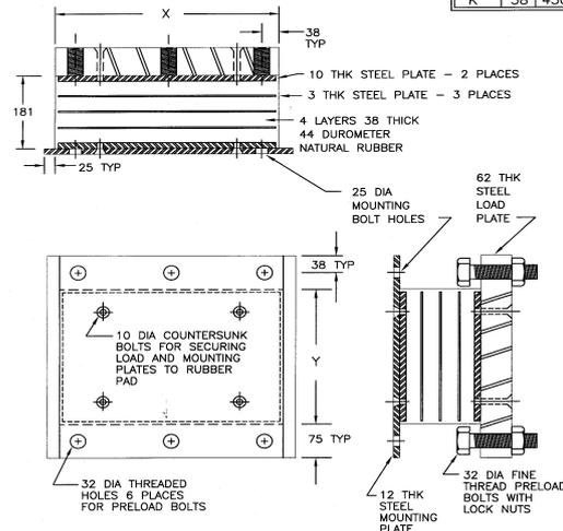
**Figure 6.** Horizontal Restraint Bearing Configuration with Provision for Preload Compression Adjustment
