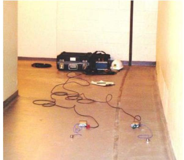
Figure 14. Vibration Measurement across the Acoustic Joint in an Exit Corridor
