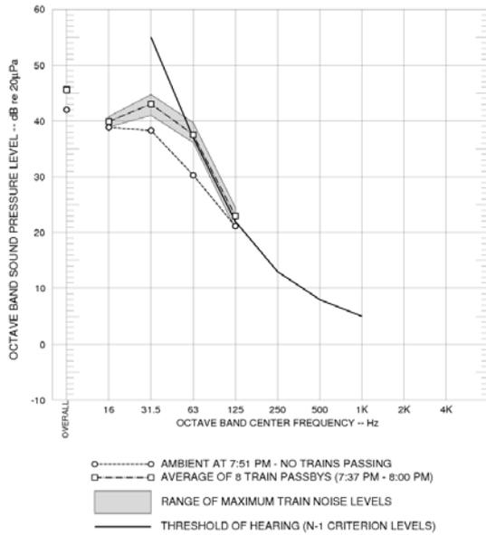
Figure 12. Maximum Noise Levels at North Aisle – Row D
