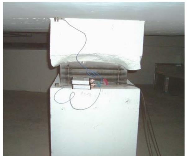
Figure 15. Vibration Measurement across the Acoustic Joint at a Foundation Element
