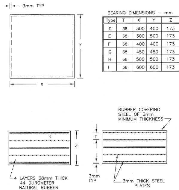
**Figure 5.** Typical Configuration for Vertical Load Rubber Isolation Bearings for Assemblies with Grout Pads Below and Above Bearing Pads
