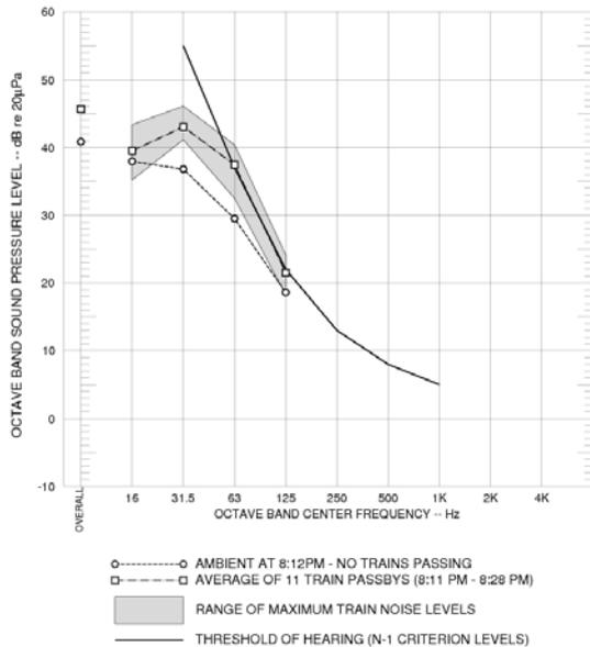
Figure 13. Maximum Noise Levels at North Aisle – Row W
