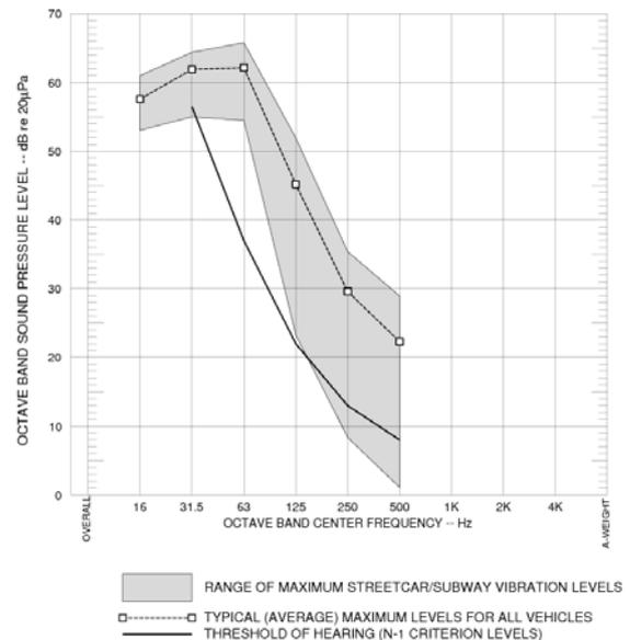
**Figure 3.** Range of Maximum Estimated Radiated Noise Levels Inside Main Hall without Isolation
