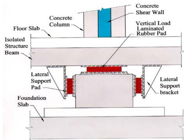
Figure 1. Essential isolation design elements
