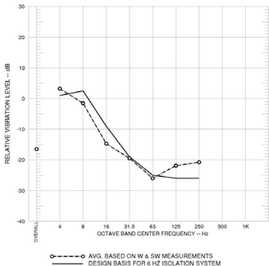
**Figure 16.** Structure/Groundborne Vibration Reduction Closest to the Subway Compared with the Design Curve
