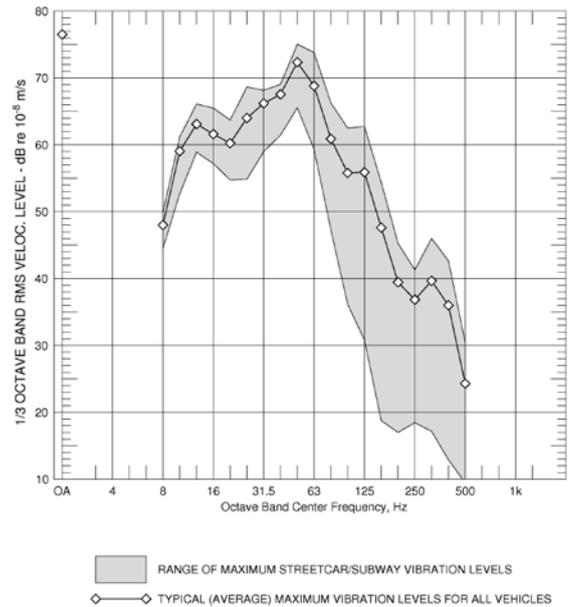
**Figure 2.** Range of Maximum Ground Vibration Levels due to Passbys of All Rail Vehicles
