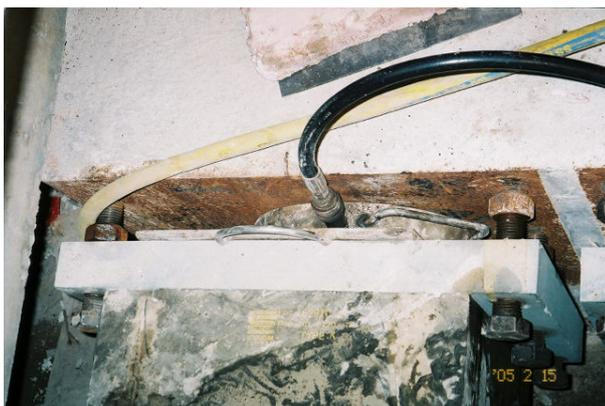
**Figure 10.** Hydraulic Jack used to preload the Lateral Pads
