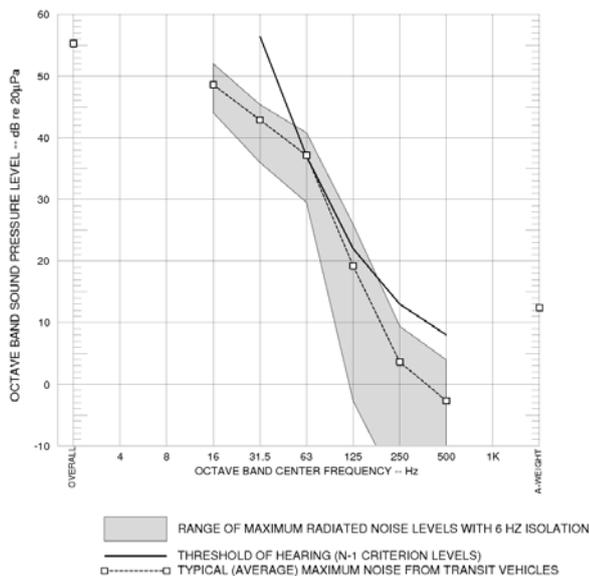
**Figure 4.** Projected Maximum Interior Radiated Noise Levels with 6 Hz Isolation System
