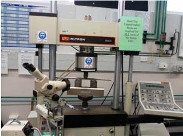
Figure 1. Experimental set-up for fatigue crack growth
