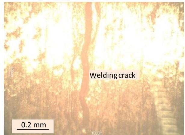
**Figure 5.** Welding crack observed under Moticam 2300 microscope.
