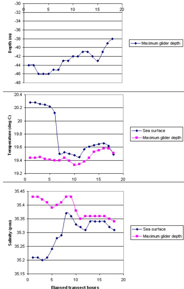
**Figure 3** Temperature, Salinity and maximum glider depth during a 20 hour transit time for glider “k90”
