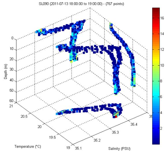
**Figure 6** 3D Temperature Salinity Water Depth diagram for 1 hour of data which displayed hysteresis. The colour intensity scale shows the number of points which recorded each temperature salinity pair
