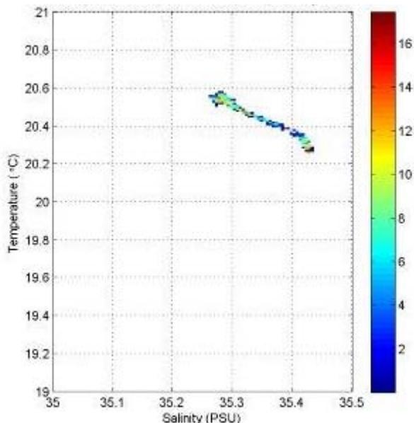
**Figure 5** TS diagram for water column with a distinct profile based on 1 hour of data. The colour intensity scale shows the number of points which recorded each temperature salinity pair
