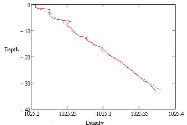
**Figure 10** Density (kg/m<sup>3</sup>) calculated for a single down and upcast from a glider measuring temperature, salinity and depth (m). The red solid curve is the downcast and the blue dotted curve the upcast
