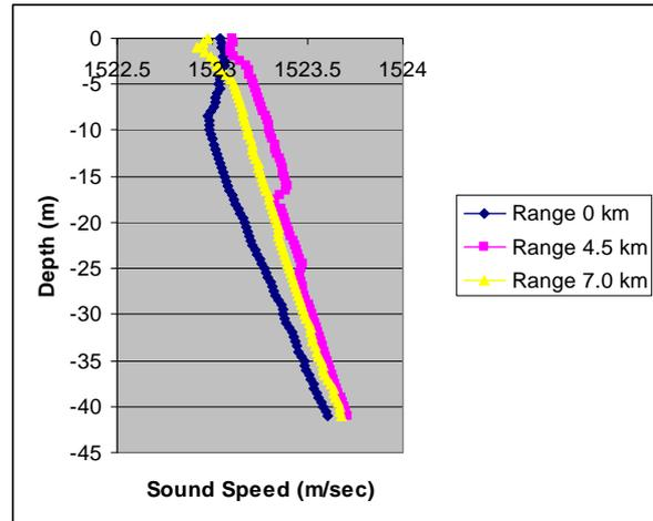
**Figure 17** Sound speed profiles based on concatenated upcast glider measurements using the raw ranges given in Figure 16
