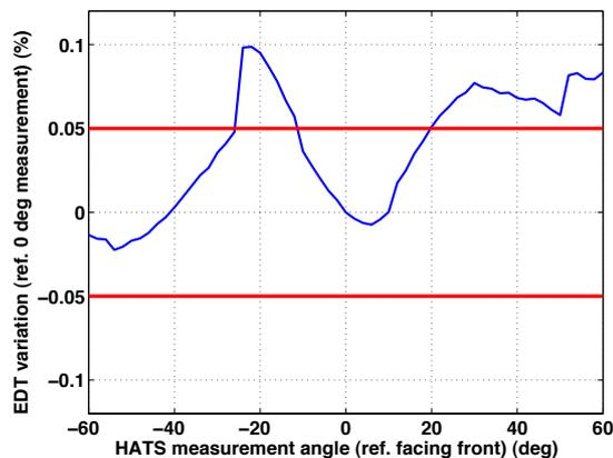
Figure 3. EDT variation for the measured OBRIRs in blue as a percentage of deviation from the 0 degree measurement. JNDs in two directions are shown in red.
