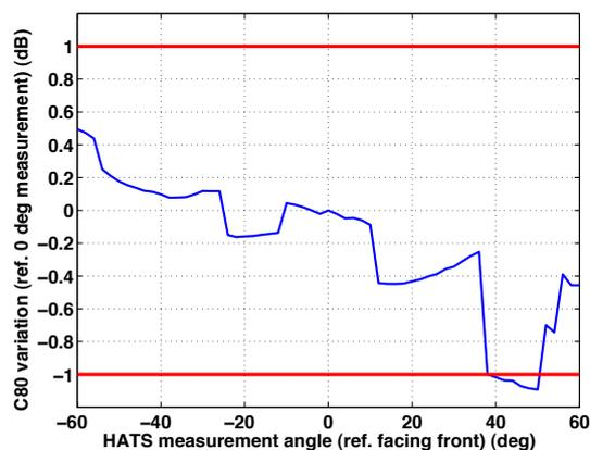
**Figure 4.**  $C_{80}$  variation for the measured OBRIRs in blue expressed as the difference in dB from the 0 degree measurement. JNDs in two directions are shown in red.
