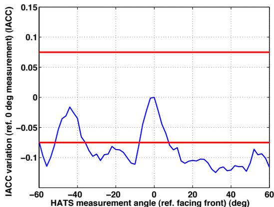
**Figure 5.** IACC variation for the measured OBRIRs in blue express as the difference in IACC from the 0 degree measurement. JNDs in two directions are shown in red.
