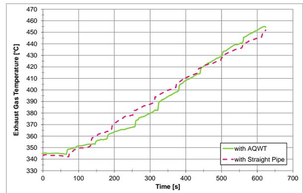
**Figure 12.** Measured EGT at M3 over time for a constant engine speed of 1800rpm, for both with an AQWT (solid line) and with a straight pipe (broken line) installed in the exhaust system. Beginning with 60kW applied to the engine, a continual load of 7kW/min was applied over 10 minutes (resulting in 130kW).
