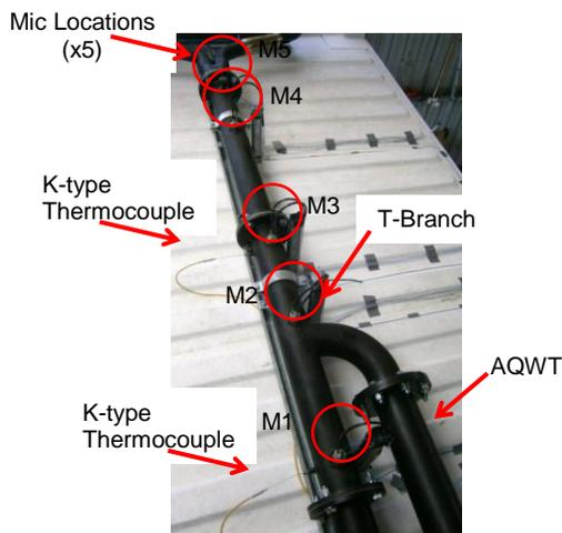
**Figure 5:** Photograph of the installed exhaust showing the side-branch and QWT, and positions of the water cooled microphones.
