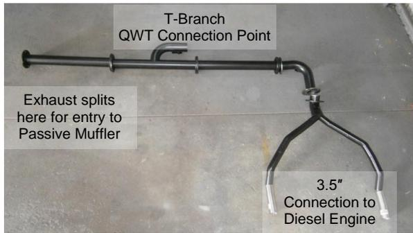
**Figure 3.** Photograph of the 4.5” (114mm) exhaust system before fitting to the Mercedes Benz diesel engine.
