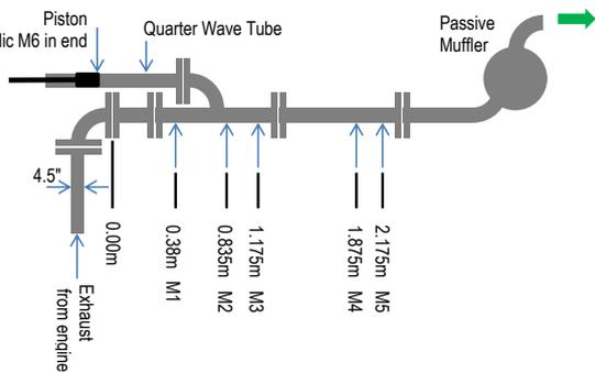
**Figure 4.** Schematic showing location of microphones mounted in the exhaust system.
