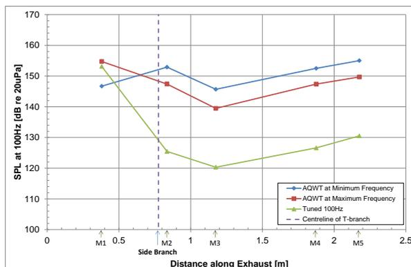
**Figure 8.** Sound Pressure Level at 100Hz for distances along the exhaust pipe for a constant engine speed of 1500rpm. No load was applied to the engine and the EGT at the side-branch was 163°C.
