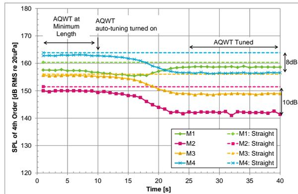
**Figure 10.** Comparison of with (solid line) and without (broken line) an AQWT installed in the exhaust system. When AQWT installed: variation from minimum length to tuned. Engine at 1500rpm, 106kW load, EGT 450°C
