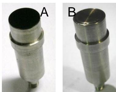
**Figure 14.** Photo of a microphone with soot on the face (A) and after cleaning (B).
