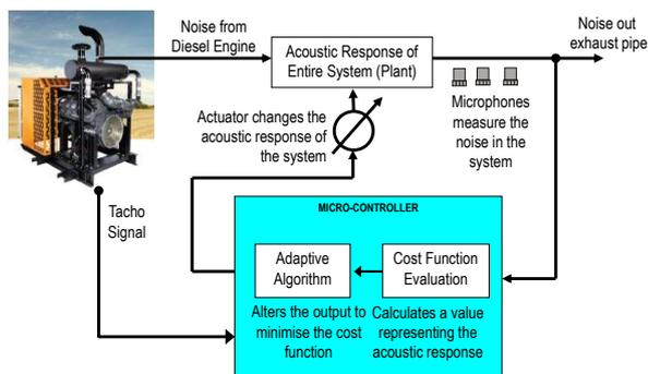
**Figure 7.** Process and control diagram for the adaptive quarter-wave tube.
