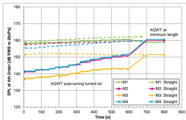
**Figure 13.** Measured SPLs over time at microphones M1 to M4 for a constant engine speed of 1800rpm. Beginning with 60kW applied load, a continual load of 7kW/min was applied over 10 minutes (resulting in 130kW). The EGT increased from 344°C to 452°C.
