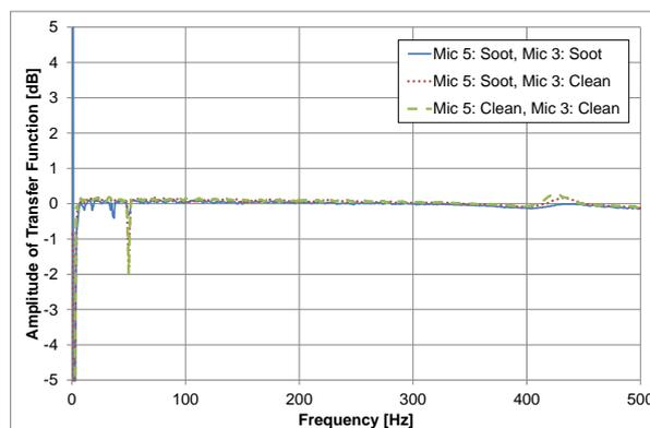
**Figure 15.** Amplitude of the transfer function between microphones with and without soot on the face.
