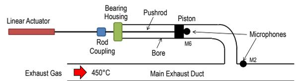
**Figure 6.** Components of the Adaptive Quarter-Wave Tube.
