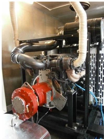
**Figure 1.** Photograph of the Taylor water brake dynamometer (red) mounted to the flywheel of the diesel engine. Also shown are the heat shielded (white) exhaust pipes.
