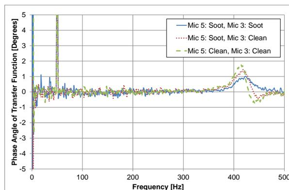
**Figure 16.** Phase angle of the transfer function between microphones with and without soot.
