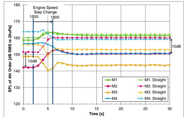
**Figure 11.** Measurement of SPL over time for a step change in engine speed from 1500rpm to 1800rpm, for both with an AQWT (solid line) and with a straight pipe (broken line) installed in the exhaust system. A constant EGT of approx. 450°C was maintained.
