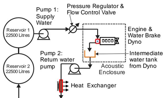
**Figure 2.** Water storage and recirculation system for dynamometer and water-cooled microphone mounts.
