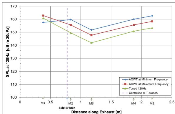
**Figure 9.** Sound Pressure Level at 120Hz for distances along the exhaust pipe for a constant engine speed of 1800rpm. A load of 125kW was applied to the engine and the EGT at the side-branch was 447°C.
