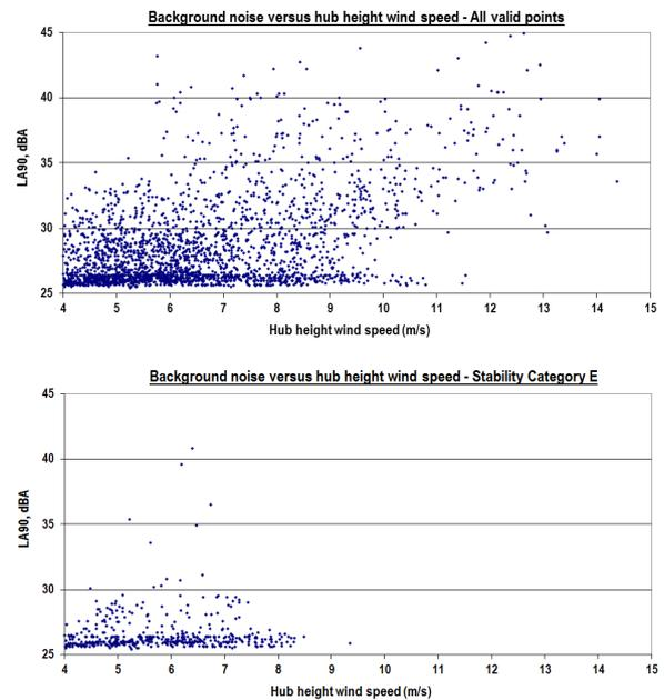
**Figure 14: Background noise levels filtered on stability conditions**
