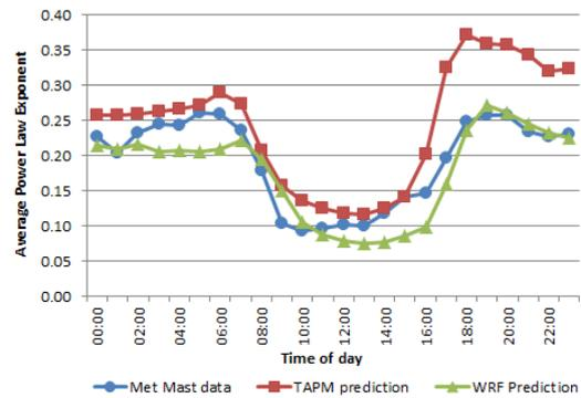
Figure 4: Stability vs. Time for a South Australian wind farm (2011 met mast data, 2008 TAPM prediction, and 2011 WRF prediction)
