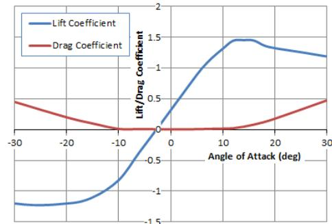
Figure 7: Lift and Drag Coefficients for typical blades
