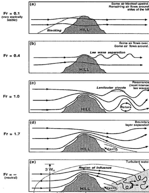
Figure 2: Idealised flow over an isolated hill (Stull 1988)
