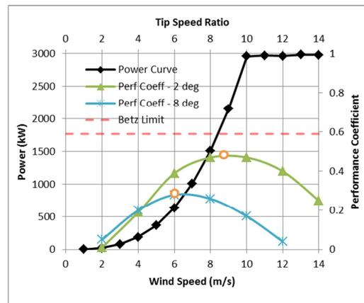
Figure 8: Variation of Power and Performance Coefficient with Tip Speed Ratio
