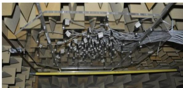
**Figure 4.** Acoustic beamformer array installed in the AWT.
