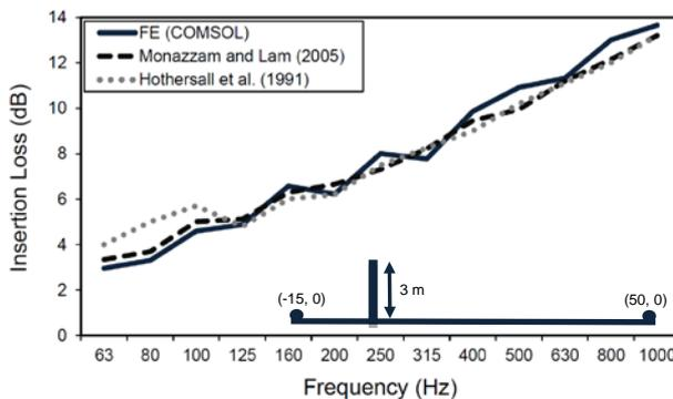
**Figure 3.** Insertion loss of a 3 m vertical barrier for the source and receiver located on the ground
