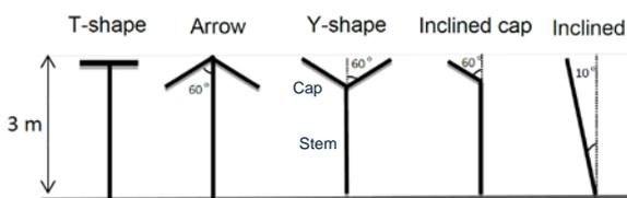
**Figure 6.** Schematic diagram of various noise barrier designs
