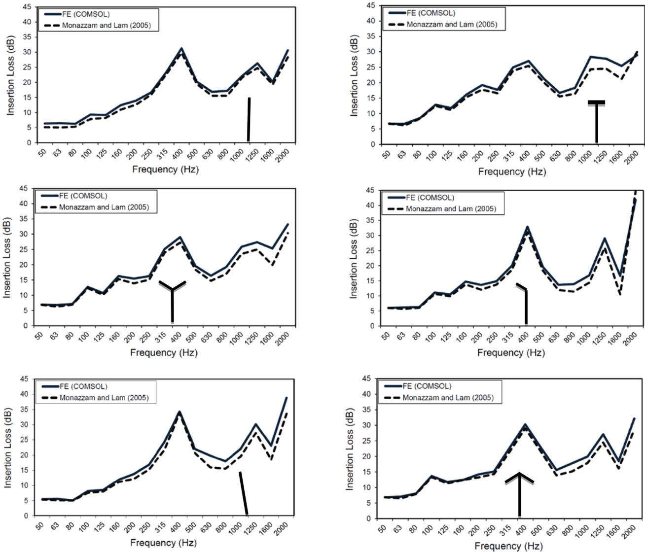
Figure 7. Insertion loss for various profiled noise barrier designs
