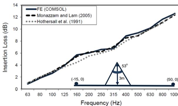
**Figure 4.** Insertion loss of a 3 m high wedge-shaped barrier
