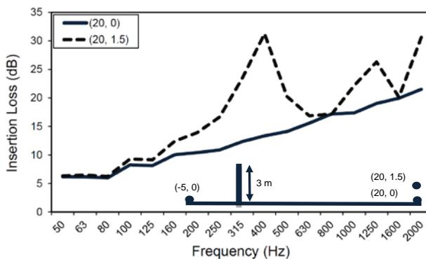
**Figure 5.** Insertion loss of a 3 m vertical barrier for different receiver heights
