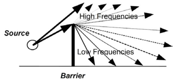
**Figure 1.** Diffraction of sound over the top edge of a barrier (Hendriks, 1998)
