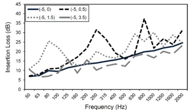
Figure 8. Insertion loss of a vertical 4 m noise barrier for various source heights
