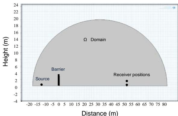
**Figure 2.** Finite element model of a vertical barrier showing the acoustic domain, source location and receiver positions
